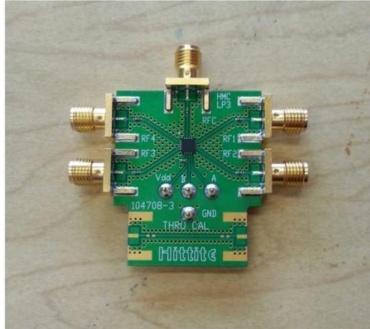
Figure 5.4 - Hittite HMC345LP3 Microwave Switch
