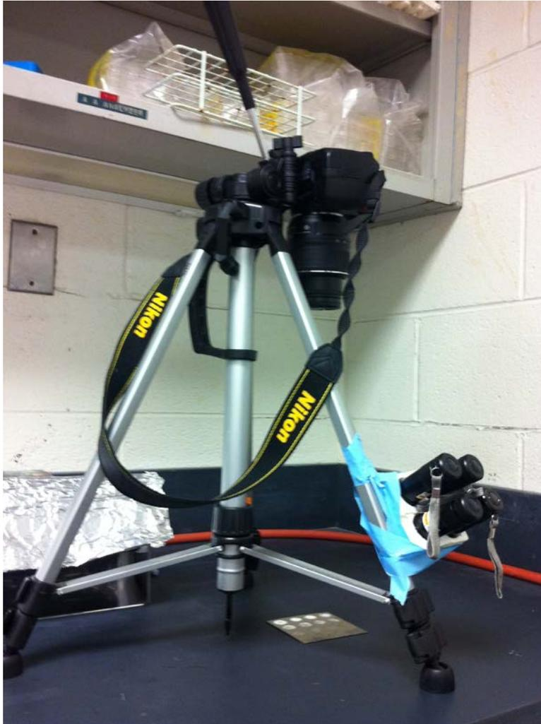
**Figure 6.8 Tripod with camera directly above sample with bundle of UV-LED lights attached to tripod stand.**
