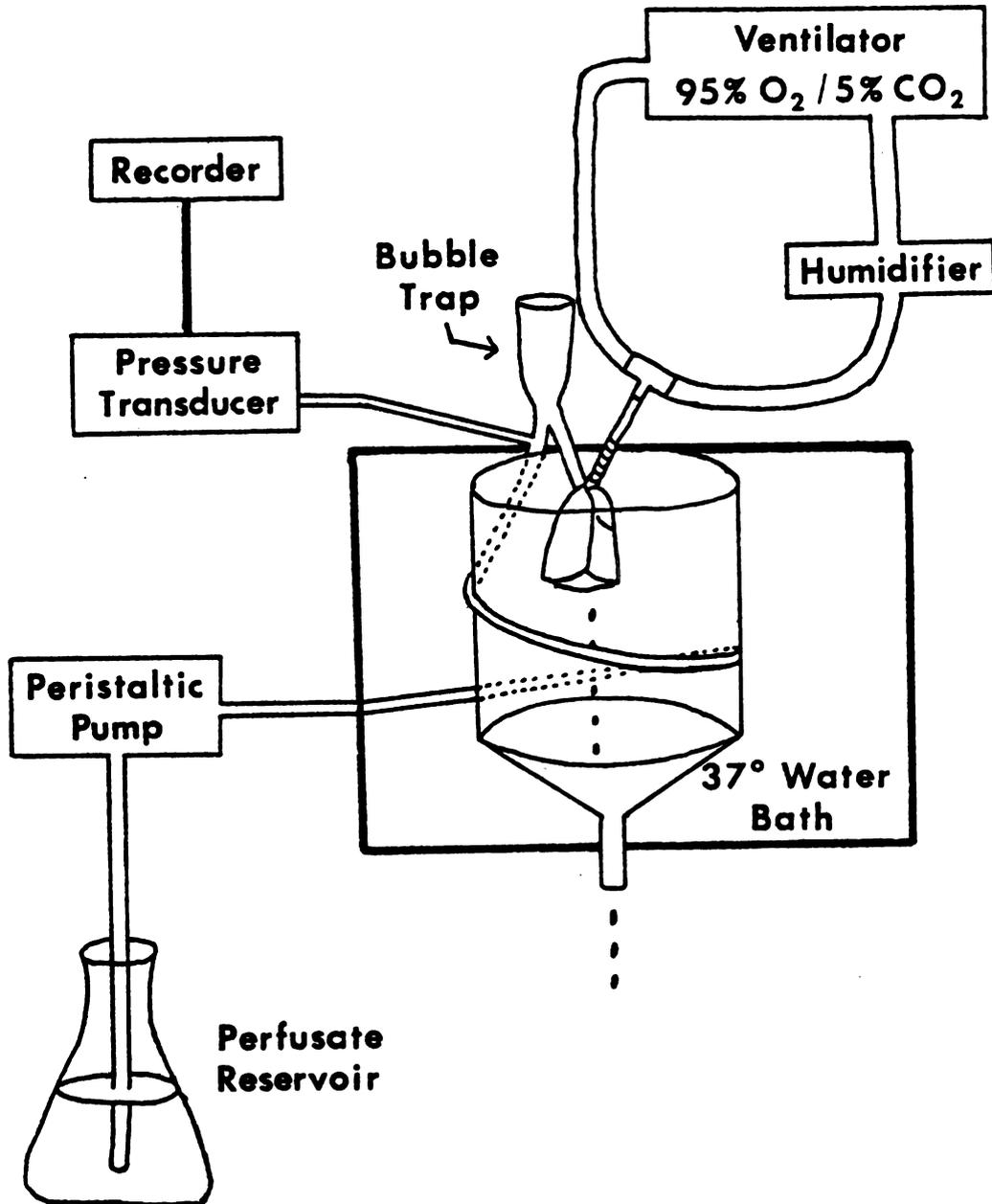
Figure 4. Diagram of isolated perfused lung preparation.
