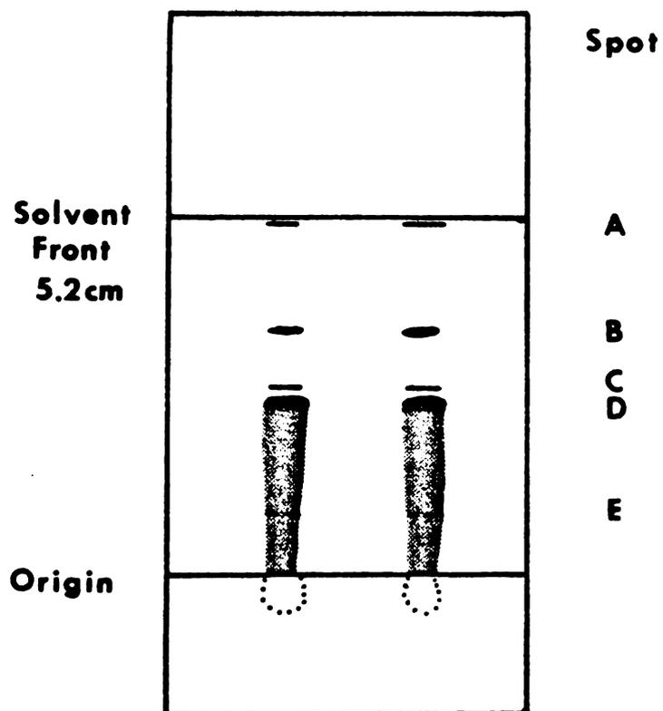
Figure 14. Diagram of TLC separation of MCTP product. Each channel was spotted with  $10\ \mu\text{l}$  of  $2\ \text{mg MCTP/ml}$  in dried diethyl ether. The plate was developed in diethyl ether: methanol : diethylamine (96.8 : 2 : 1.2). Spots were detected by spraying with Ehrlich's reagent followed by heating.
