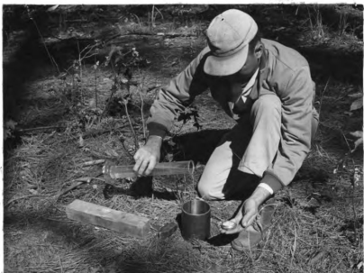
Fig. 11.-Pouring water into infiltration tube and measuring time of infiltration.
