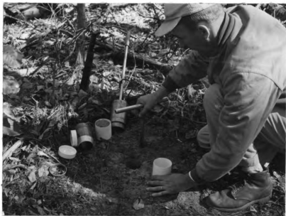
Fig. 9.-Thrusting 1-inch sampler tube 3 inches into topsoil to obtain portion of composite sample.
