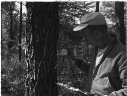
Fig. 12.-Using a dial gauge micro-dendrometer to measure radial growth of a loblolly pine.
