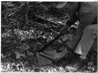
Fig. 3.--Cutting the forest floor sample. The plywoodboard is 1 foot square.
