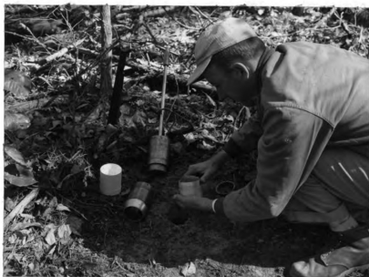
Fig. 8.-Rough-trimming the base of the volumetric sample with a hunting knife. Cylinder and sample fit snugly into the ice cream container.
