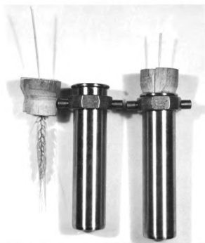
Figure 6. Tapered wood plugs and metal test cups used to mount wheat heads in a commercial centrifuge
