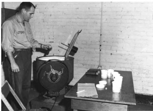
Figure 7. Commercial centrifuge used for exploratory centrifugal threshing
