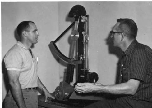
Figure 12. Straw tensile strength was determined by use of Schopper testing machine.
