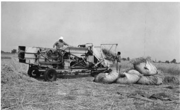
Figure 15. Straw discharged over the rack was analyzed to determine rack and cylinder losses by use of a rethresher.
