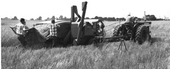
Figure 14. Canvasses were used to collect total discharge from the rack during field combine tests.
