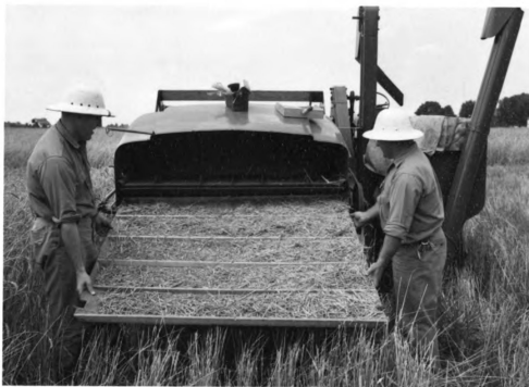
Figure 17. Grain and straw passing through the rack was collected by a wooden tray with five zones inserted under the rack.
