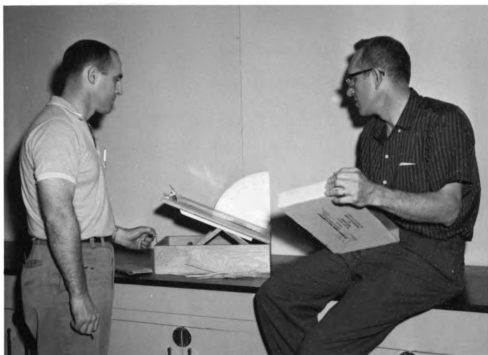
Figure 13. Straw frictional data were obtained with a tilting board device, surfaced with galvanized metal.
