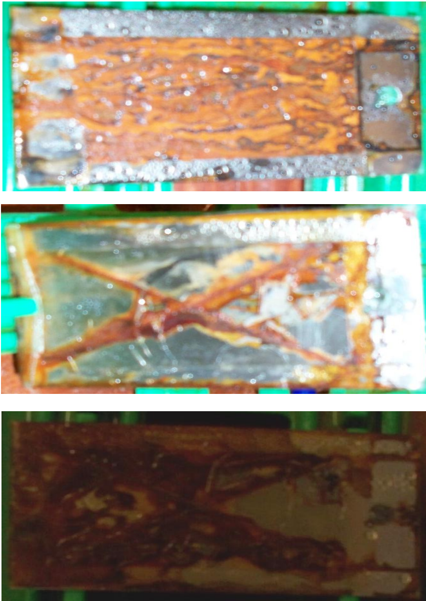
Figure 6.22 Panels after 91 hours in salt spray. Blank (Top), Coated -no corrosion inhibitor (middle) and Coated - 3% corrosion inhibitor (bottom)
