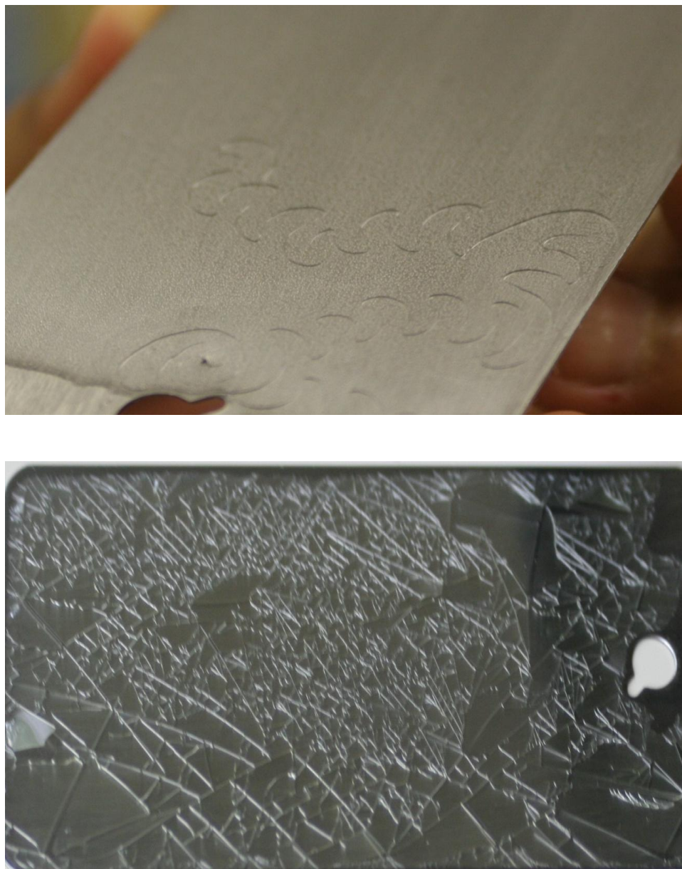
Figure 6.19 Initial cracking (Top) and complete cracking (bottom) of panel coated with 1:15 silylated oil, 0.5 phr DBTDL
