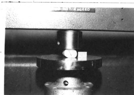
Fig. 7-1 Crack just initiated at the center of a potato sample
