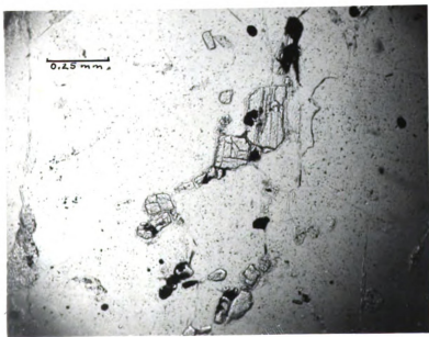
Figure 29. Andalusite filling interstices between quartz grains, McCaslin formation (Sample 51).
