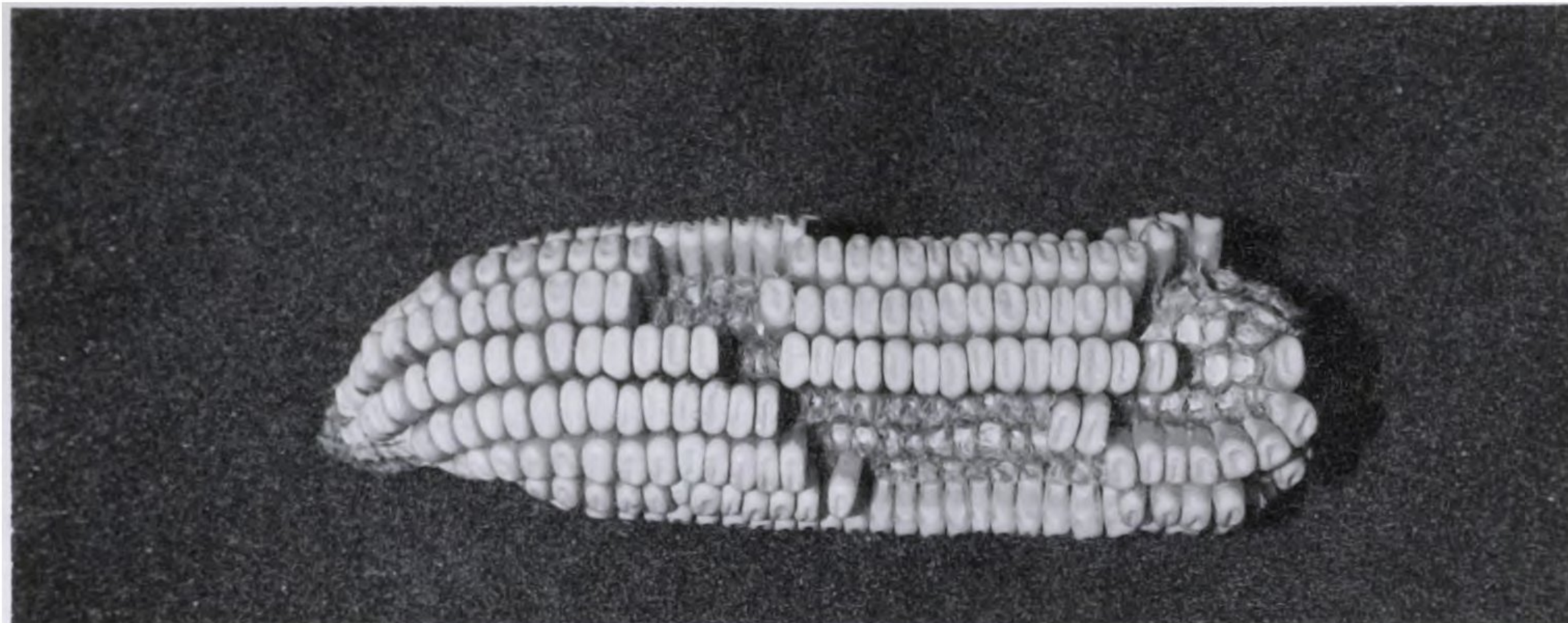
FIGURE 5.1 TYPICAL SHELLING PATTERN FROM LOW-VELOCITY IMPACT AT LOW AND MEDIUM MOISTURE LEVELS.
