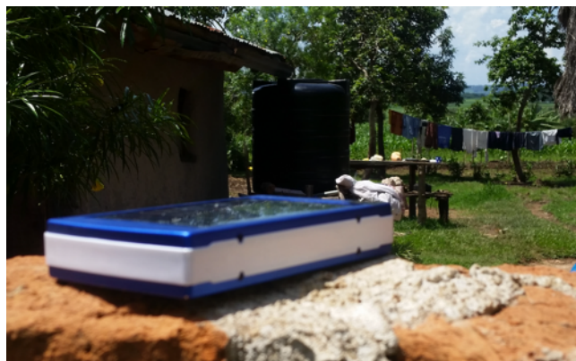
Figure 8: This figure shows an example of how participants who did not have grid electricity in their homes charge solar batteries to power M-Kulinda. This data was collected in May 2017 in Bungoma County, Kenya
