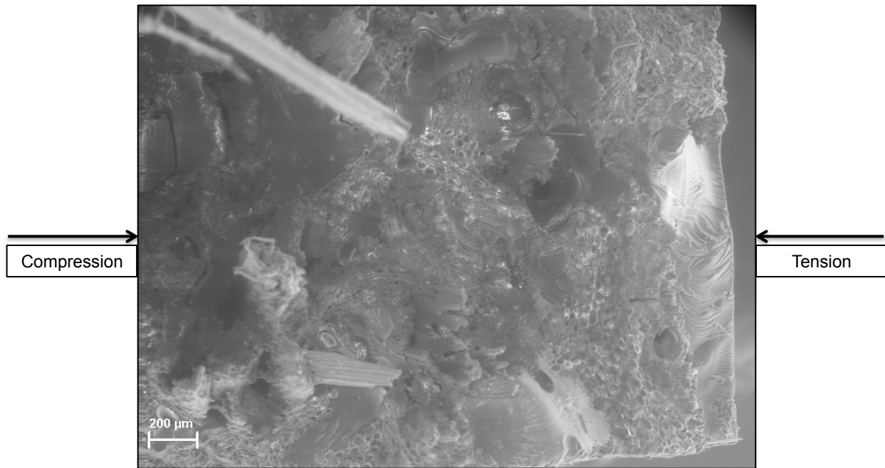
Figure 4.23 Hybrid composite 20%/20% AFEX/Basalt on tension edge. Bamboo fibers have failed by break. River patterns on resin surface.
