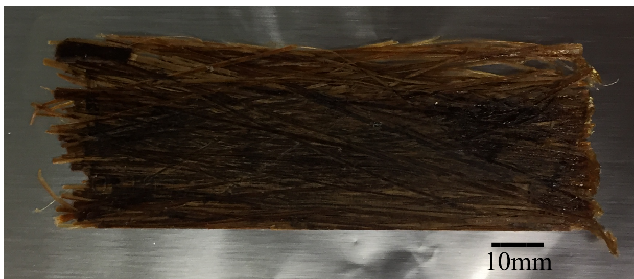
Figure 5.3 Compression-moulded Acrodur-950L (BASF) resin with AFEX-treated bamboo fibers.
