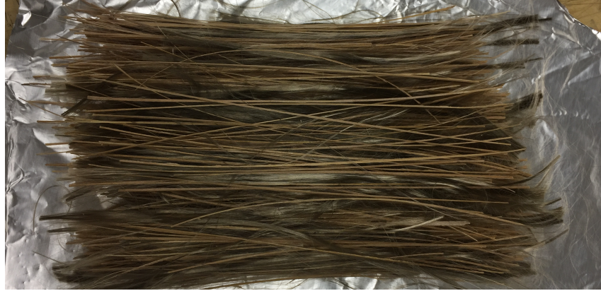
Figure 4.4 Basalt and bamboo fibers intertwined and cut to a length of 12.7 cm.
