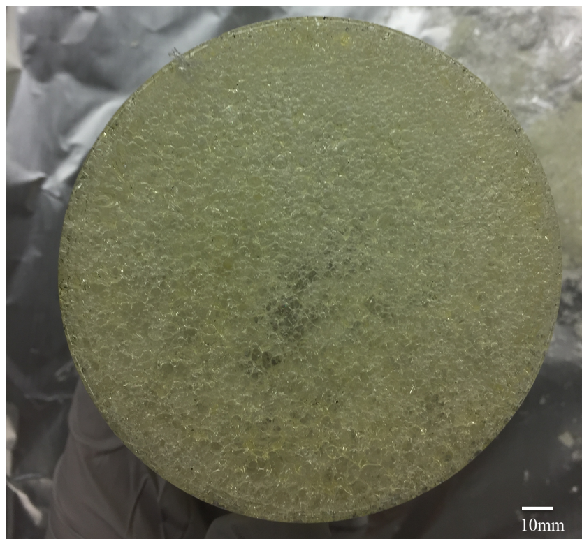
Figure 5.2 Foam structure of neat Acrodur 950L (BASF).
