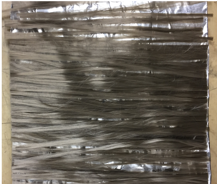
Figure 4.3 Basalt fibers cut to a length of 12.7 cm.
