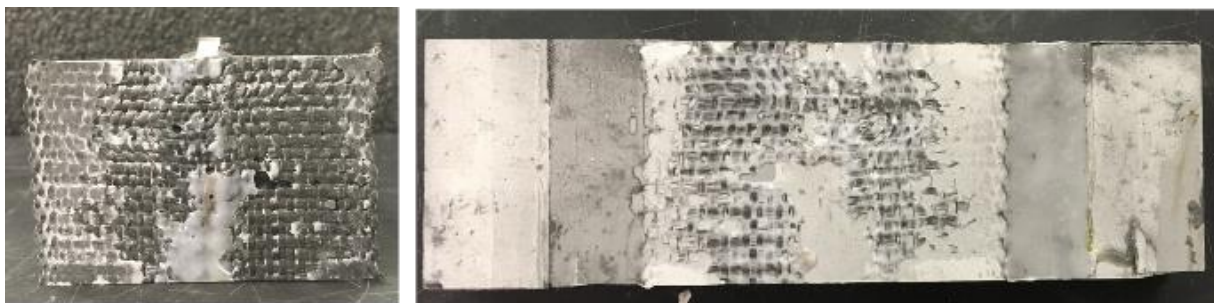
Figure 6-10. Specimen A-1 failure condition. Left-preform's surface, Right-base's surface.
