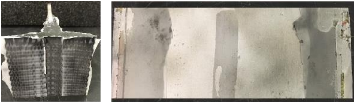
Figure 6-18. Specimen B-1 failure condition. Left-preform's surface, Right-base's surface.
