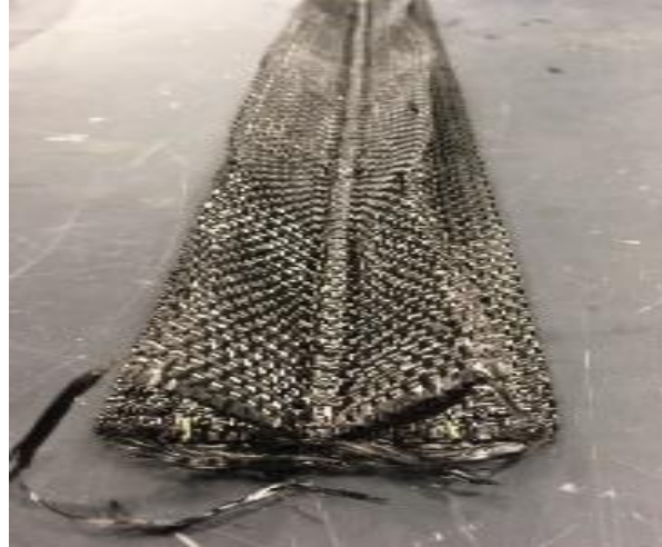
Figure 3-3. 3-D braided carbon fiber preform (Albany Composites, Inc.)
