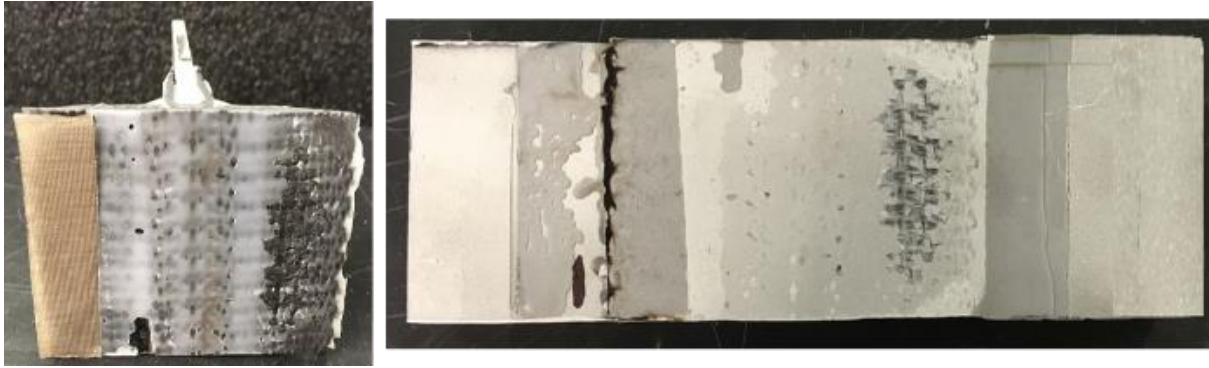
Figure 6-22. Specimen C-1 failure condition. Left-preform's surface, Right-base's surface.
