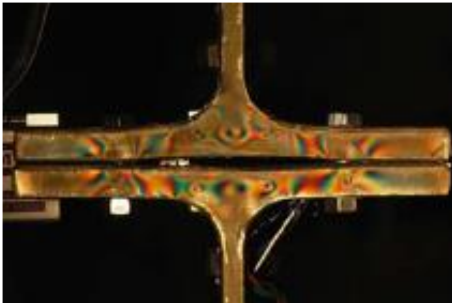
Figure 2-11. The isochromatic whole-field strain fringe pattern of bolted T-stub joints [5]
