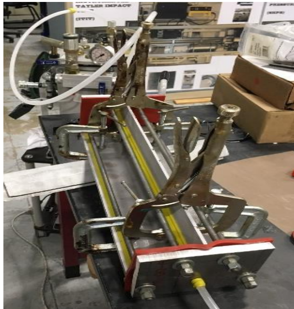
Figure 3-5. Completed assembly for manufacturing aluminum pi-joints
