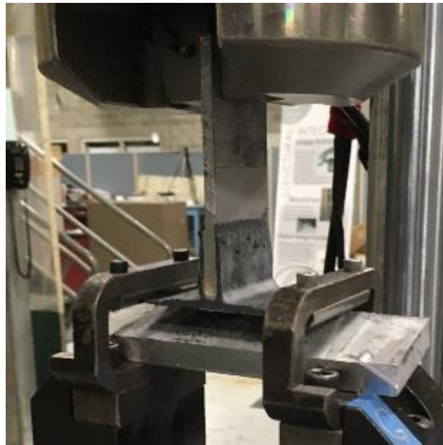
Figure 6-9. Complete separation of the base from preform during the pi-joint pull-out test.
