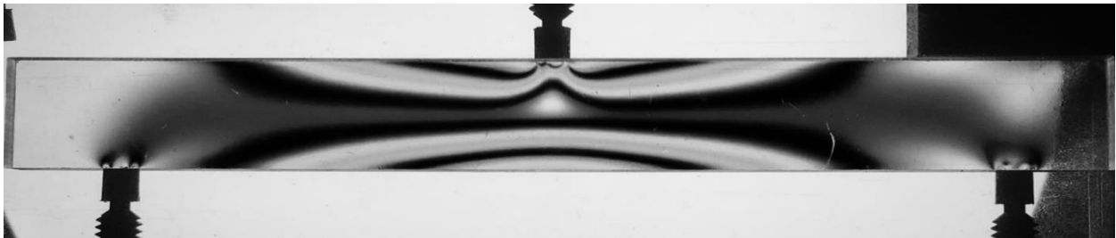
Figure 1-1 Isochromatic fringe photoelasticity pattern on a polycarbonate block in a 3-point bending loading
