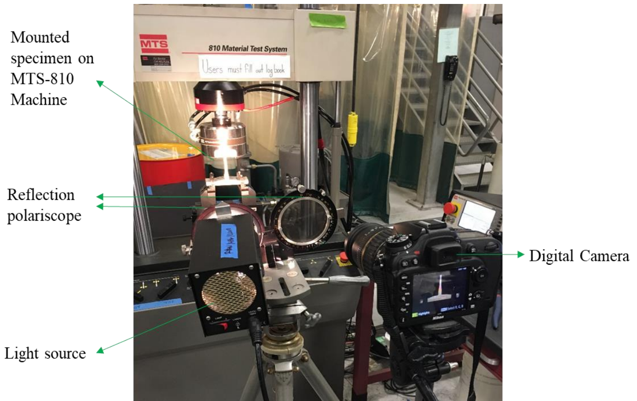
Figure 4-3. Experimental Test Setup
