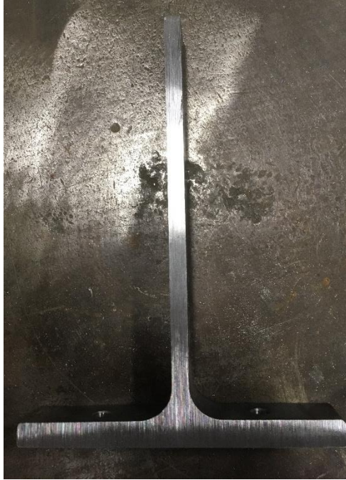
Figure 4-4. Steel T-joint specimen with 24 mm thickness.
