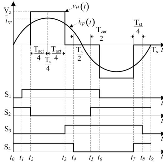
Figure 4. 3 ZSRC H-bridge output voltage, primary side resonant current, and PWM waveforms (phase shift control)
