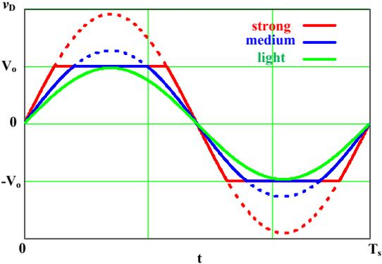
Figure 5. 5 Secondary side waveform in one switching period with different excitations
