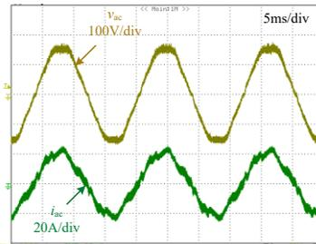
(c) Proposed input power approach, pulse notch control @full load
