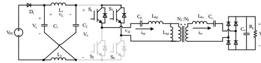
(g) Normal zero state,  $t_4 \sim t_5$
