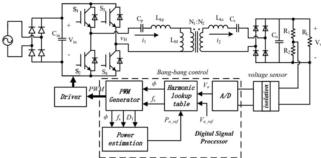
Figure 3. 5 Control diagram for harmonic burst
