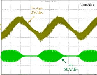
(c) Secondary side output voltage ripple
