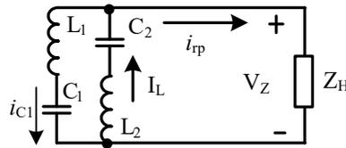
Figure 4. 11 Equivalent circuit in output voltage discontinuous mode
