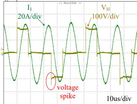
Figure 3. 11 Experimental waveforms of PFM @Full load
