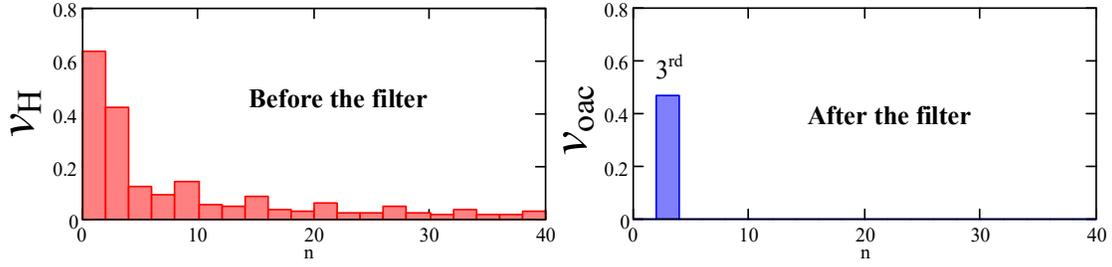
Figure 2. 4 Harmonic component of  $v_H$  &  $v_{oac}$  ( $D=0.33$ , filter  $R_{ac}=\omega L_M$  in Figure 2. 2, 3<sup>rd</sup> harmonic selected as an example)
