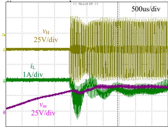
(b) Startup at the rising edge of the AC voltage
