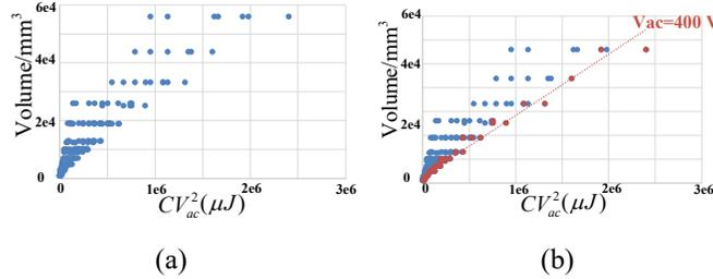
Figure 2. 13 An example of capacitor volume-energy map from KEMET R73 series capacitors
