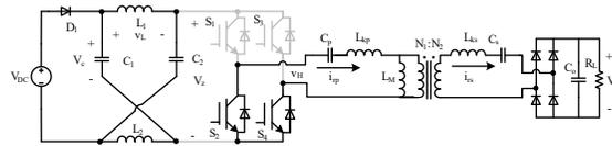
(h) Normal zero state,  $t_0 \sim t_1$  &  $t_8 \sim t_9$
