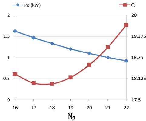
Figure 2. 9 Maximum power and quality factor curve vs. secondary turns  $N_2$  (@ $V_{in}=190$  V,  $N_1=5$ ,  $R_o=40$  Ohm)
