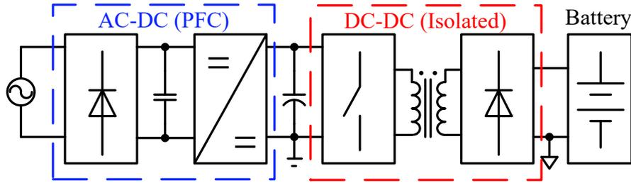
Figure 1. 2 Block diagram of a conventional OBC
