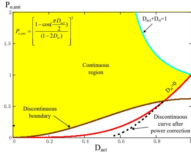
Figure 4. 13 Unified power curves for pulse notch control with power correction
