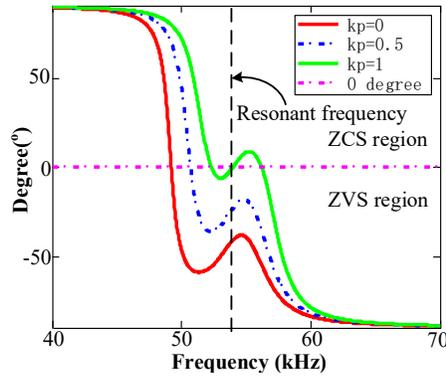
Figure 2. 8 Primary side current phase of H-bridge vs. frequency with different  $k_p$  @ $k_s=1$
