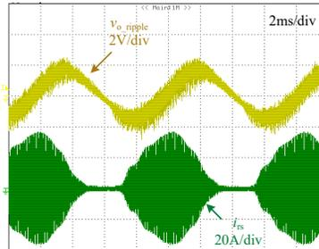
(c) Secondary side output voltage ripple
