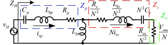
Figure 5. 4 A simplified circuit of the resonant network
