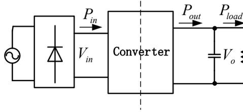
(a) Power flow in circuit diagram
