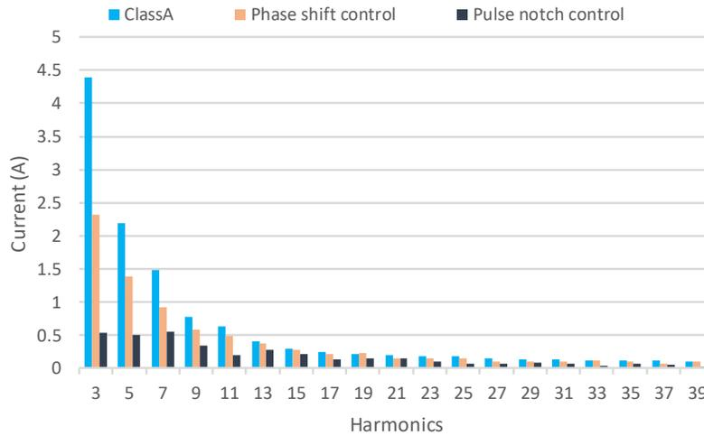
Figure 5. 15 Input current spectrum at half load (200 V/500 W)
