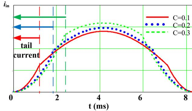
Figure 5. 8 Input current waveform with different constant C
