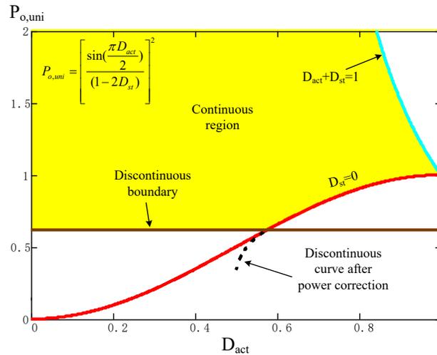
Figure 4. 14 Unified power curves for phase shift control with power correction
