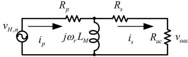
Figure 3. 8 Equivalent simplified circuit for SRC at resonant frequency (N=1)
