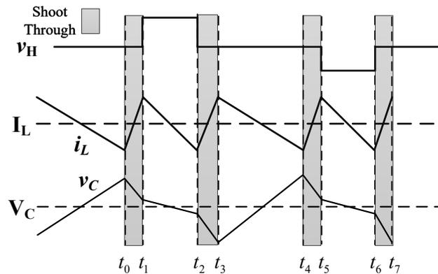
Figure 5. 12 Z-source inductor current and capacitor voltage in one switching period
