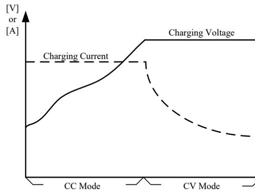
Figure 1. 5 On-board battery charger (OBC) charging mode
