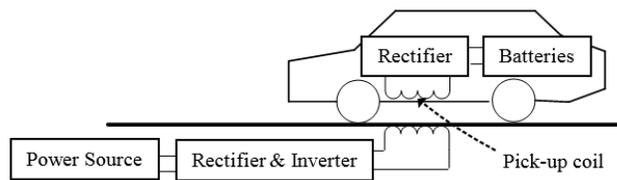
Figure 1. 1 Configuration of a wireless power transfer system for OLPT
