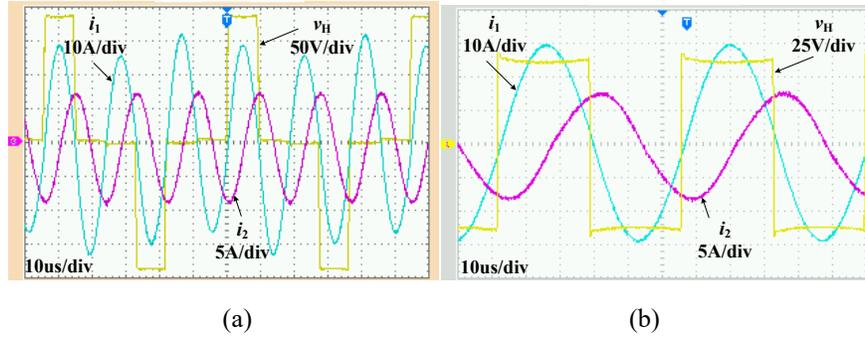
Figure 2. 15 Experimental waveforms for third harmonic system (a) and for fundamental system (b) @ $R_o=40$  Ohm
