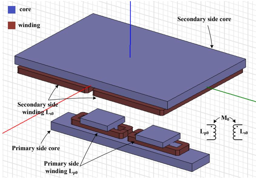
Figure 2. 5 FEA model for transformer
