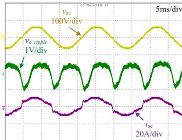
(c) Secondary side output voltage ripple
