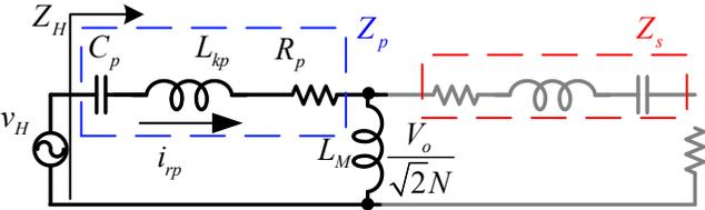
Figure 5. 6 A simplified circuit of the resonant network at power discontinuous mode
