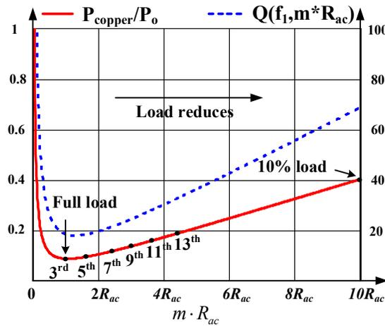
Figure 3. 7 Copper loss to output power ratio vs. output load at resonant frequency without regulation (open loop)
