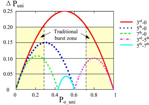
Figure 3. 10 Unified pulsed power vs. unified output power in harmonic burst control
