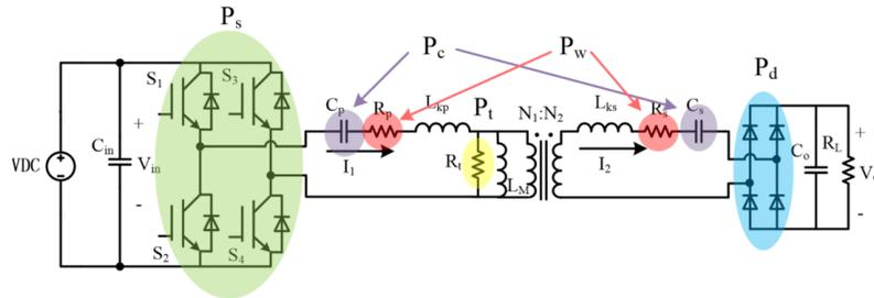
Figure 2. 10 Schematic diagram for conventional IPT prototype
