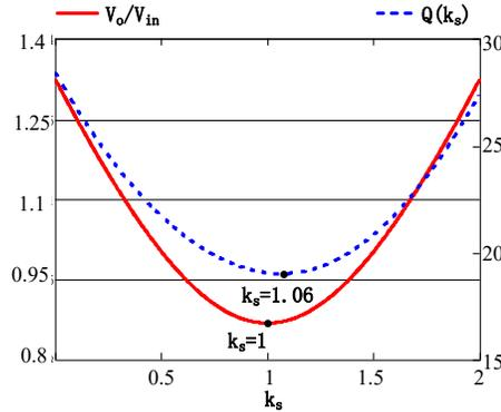
Figure 2. 7 Voltage gain and quality factor curves vs.  $k_s$  with resistive impedance ( $Z_{H2}$ ) constrain and fixed turns ( $N_1=5, N_2=20$ )
