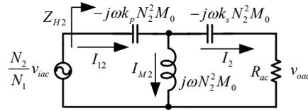
(a) Resonant LCs are replaced by short circuit
