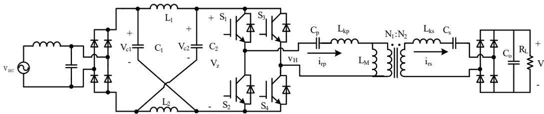
Figure 4. 1 Circuit schematic of the proposed Z-source wireless charger
