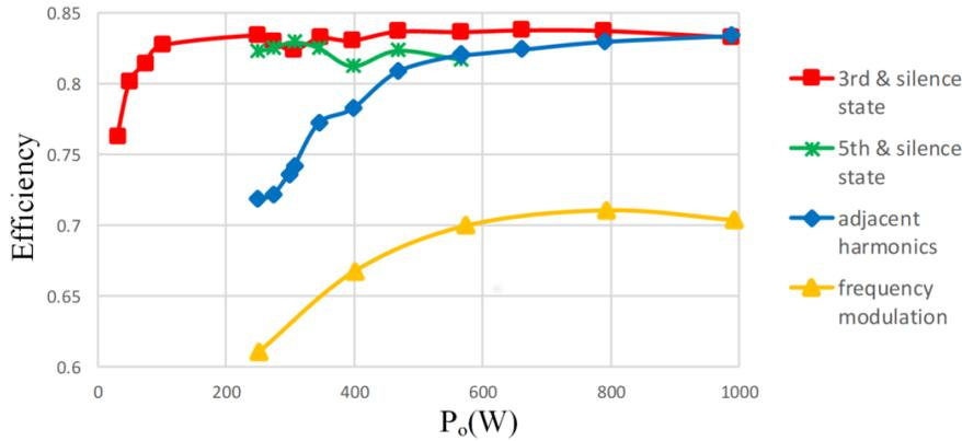
Figure 3. 15 Experimental result of efficiency with different regulation method
