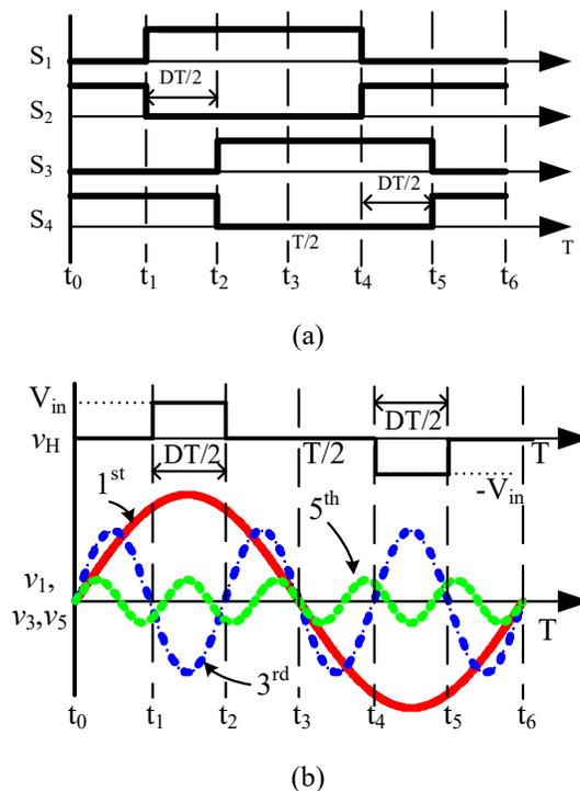
Figure 3. 1 PWM waveforms, H-bridge output voltage  $v_H$ , and H-bridge output voltage harmonics
