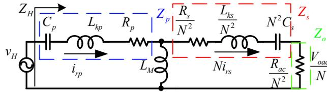
Figure 4. 8 A simplified circuit of the resonant network
