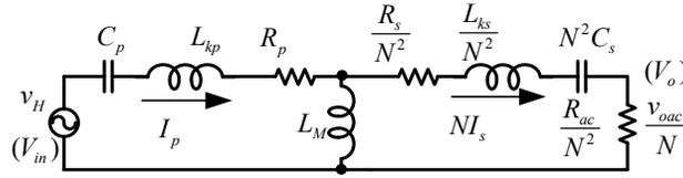
Figure 3. 6 Equivalent simplified circuit for SRC
