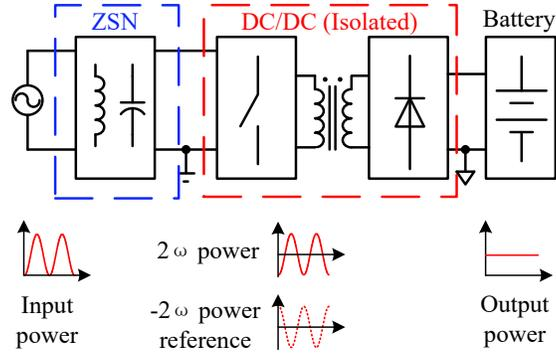
Figure 5. 2 Illustration of  $2\omega$  ripple power rejected control
