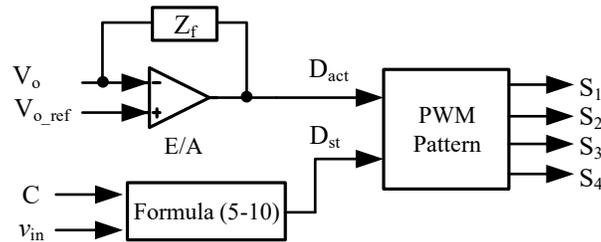
Figure 5. 9 block diagram of input current control
