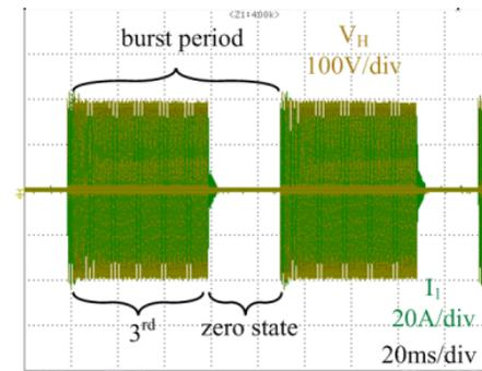
Figure 3. 13 Experimental waveforms of burst between 3<sup>rd</sup> harmonic and “silence state” @66% load
