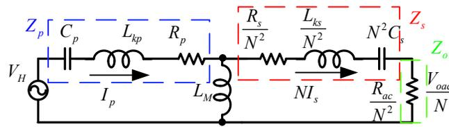
Figure 4. 4 A simplified circuit of the resonant network.
