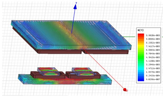
Figure 2. 11 FEA simulation result, magnetic flux plot on cores
