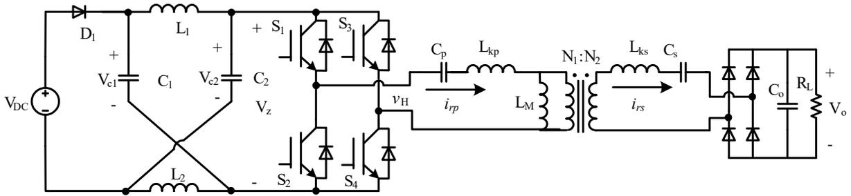
Figure 1. 6 Circuit schematic of the ZSRC
