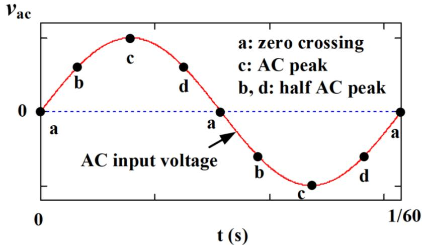
Figure 5. 20 Four candidates of soft startup instant in one line cycle
