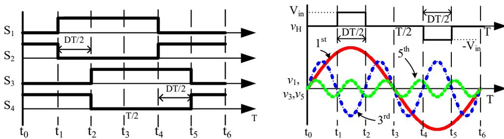
Figure 2. 3. PWM waveforms, H-bridge output voltage  $v_H$ , and H-bridge output voltage harmonics
