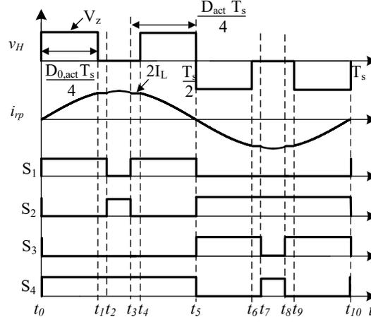
Figure 4. 12 Time domain waveforms in discontinuous mode for pulse notch control
