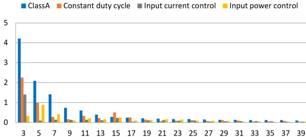
Figure 5. 19 Input current spectrum at full load (200 V/1 kW)
