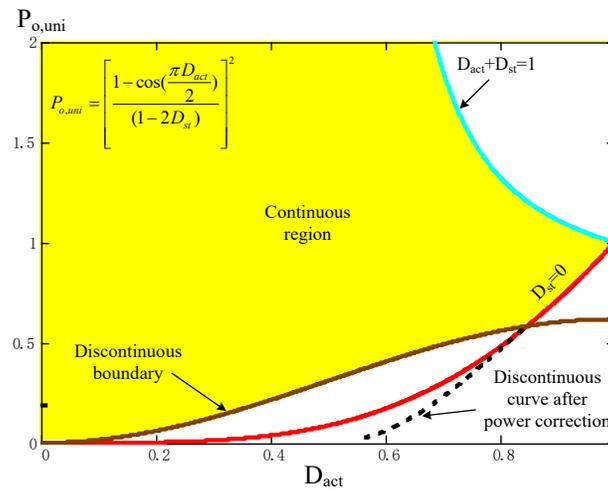
Figure 5. 1 Unified power curves for pulse notch control with power correction
