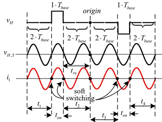
Figure 3. 4 H-bridge's output voltage and current of the full bridge inverter when passing through 5<sup>th</sup> harmonic (k=2)
