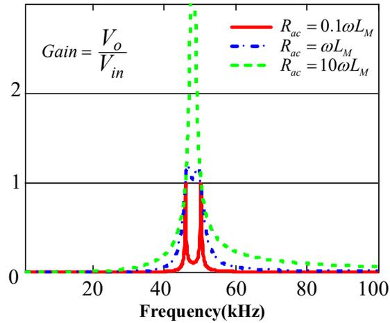
Figure 2. 2 Gain curve of IPT with different load ( $R_{ac}=0.1\omega L_M$ ,  $\omega L_M$  and  $10\omega L_M$ )
