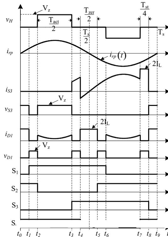
Figure 4. 5 Time domain waveforms for phase-shift control in ZSRC
