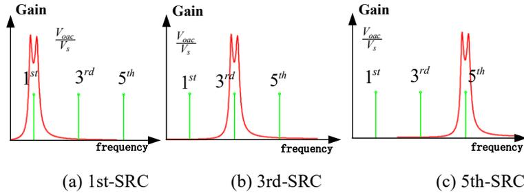
Figure 1. 4 Output to input voltage gain curves vs. frequency
