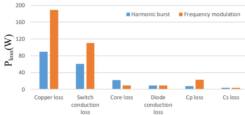
Figure 3. 16 Calculation result of loss break down with different regulation method at full load
