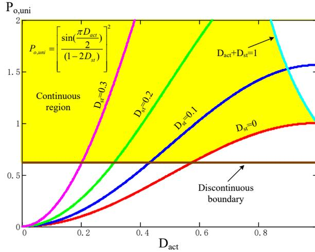
Figure 4. 9 Unified power curves for phase shift control
