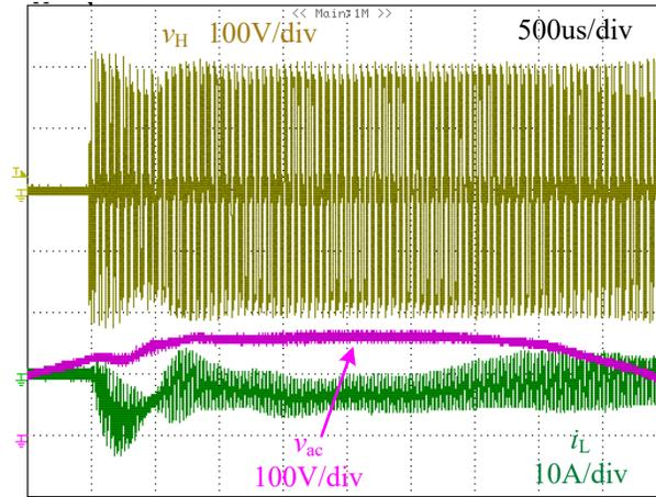
Figure 5. 22 Soft startup waveforms for the proposed input power control at full load (120 Vac/1 kW)
