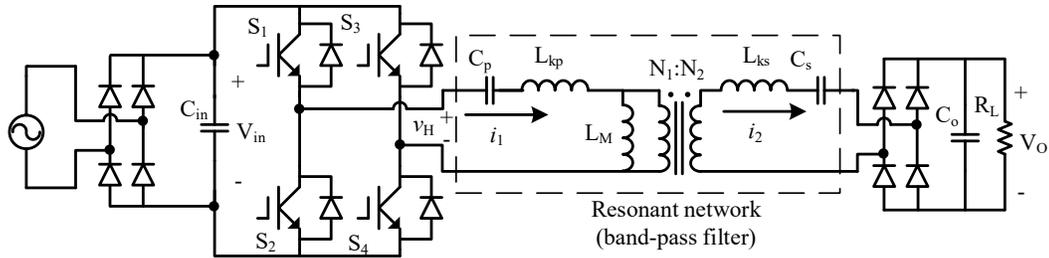
Figure 1. 3 Overall schematic diagram for the conventional IPT prototype
