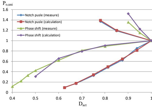
Figure 4. 19 Experimental unit power curve ( $R_L=40$  Ohm, open loop, unit power=150 W)
