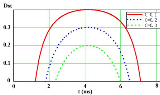
Figure 5. 7  $D_{st}$  in half line period with different constant  $C$
