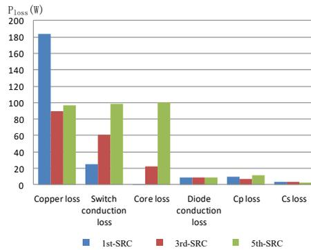
Figure 2. 12 Loss breakdown of the three IPT systems
