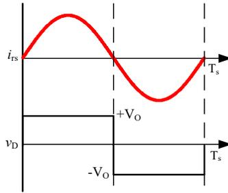
Figure 5. 3 Secondary side waveform in one switching period
