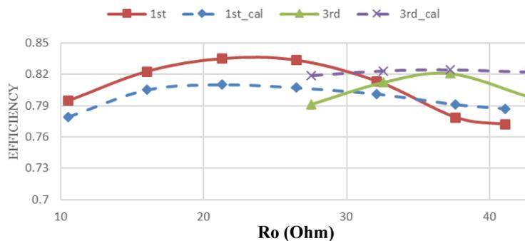
Figure 2. 16 Efficiency curve for the 1st-SRC and 3rd-SRC with different output resistances (fixed load 1-kW)
