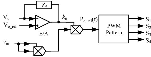
Figure 5. 10 block diagram of input power control
