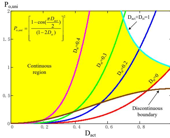
Figure 4. 10 Unified power curves for pulse notch control
