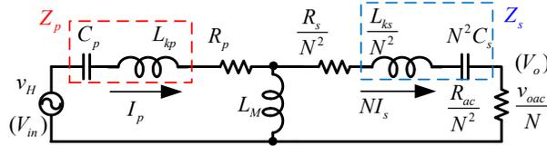
Figure 2. 1 Equivalent simplified circuit for IPT
