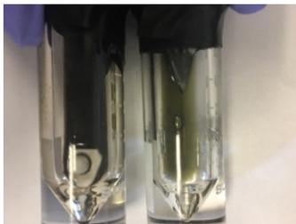
**Figure 17. Color difference after 18 h: (Right) with Hg, (Left) without Hg**
