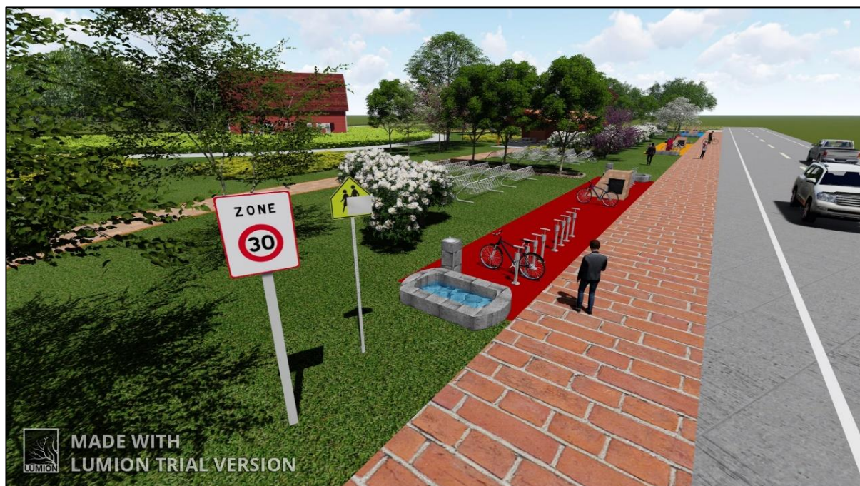
Figure 5.1 This diagram show the details of advanced bicycle landing area and an express bike service station. The brick pattern indicate the area for landing. For the express bike station, colorful pavements indicate different functions of the repair service on Site A. Therefore, cyclists can observe further away to decide if there is a need for services, the turning in action will be safer and smoother with the wide landing zone. Copyright © 2018 Yinliang Li, all rights reserved, used by permission.
