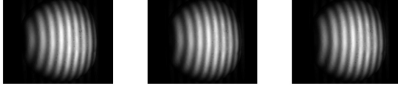
Figure 3.6. Examples of three phase-shifted pattern images of an apple, obtained under the illumination of sinusoidal pattern with phase offsets of -2\pi/3 , 0 and 2\pi/3 (from left to right), respectively.
