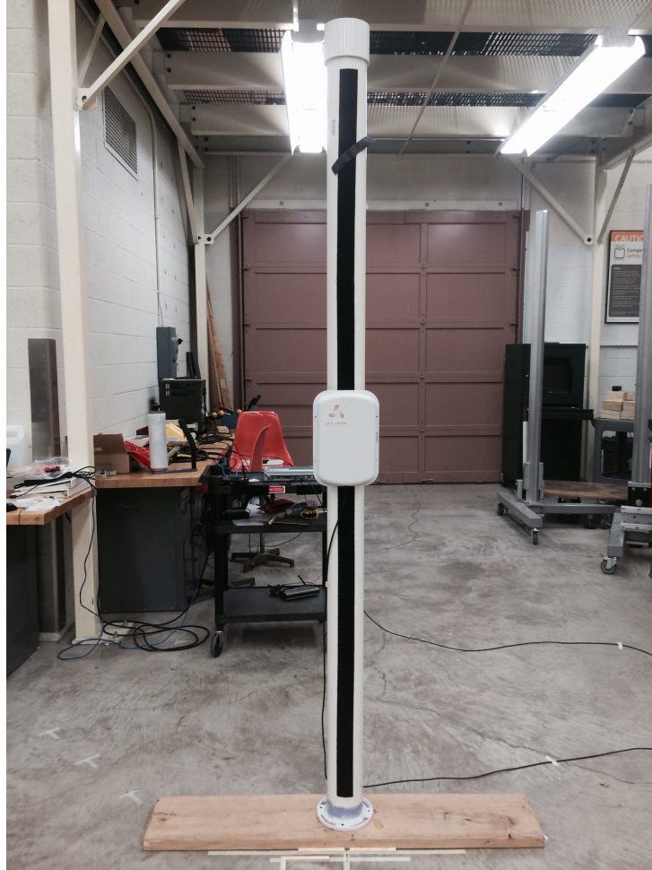
Figure 6 Circularly Polarized Antenna on the PVC Pipe.
