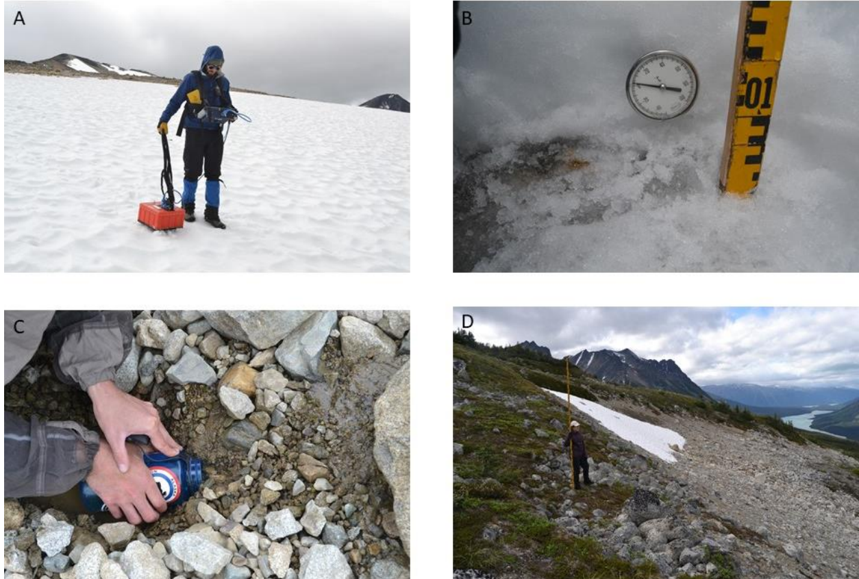
Figure 2.4. Study methods at Frost Ridge, BC: A) GPR survey of snowbanks. B) Measurements of snow temperature and density. C) Collection of suspended sediment at the downslope edge of a snowbank. D) Survey of snowbanks, surrounding topographic depressions, and periglacial features.
