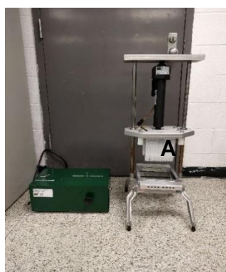
Figure 2-2: Components of NEMCO model # 59155491 stationary slicer: (A) pusher, and (B) blade
