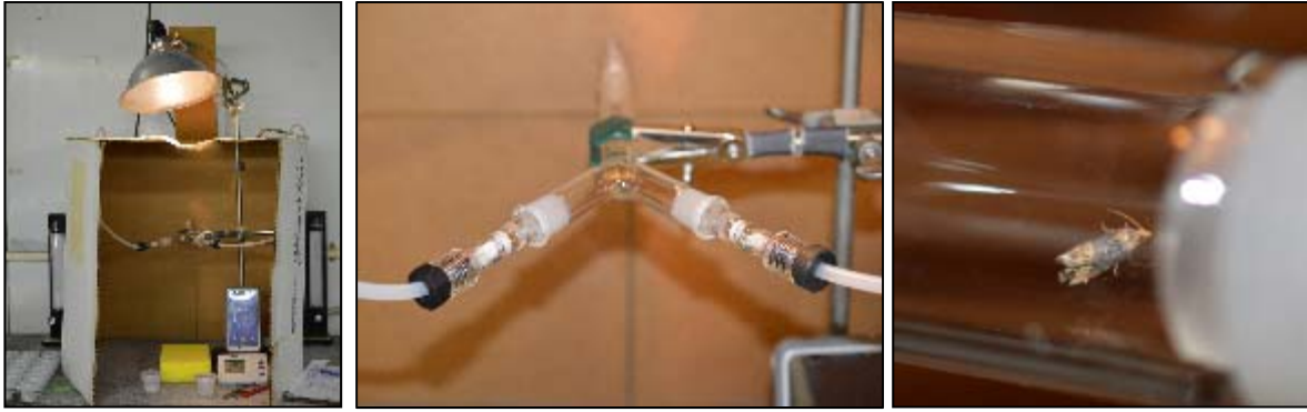
Figure 2.1. Y-tube apparatus to test behavioral responses of male P. viteana to a standard pheromone blend or to females from different populations. Left) Y-tube set up showing experimental enclosure; middle) close-up of Y-tube; right) male moth in one arm of the Y-tube.
