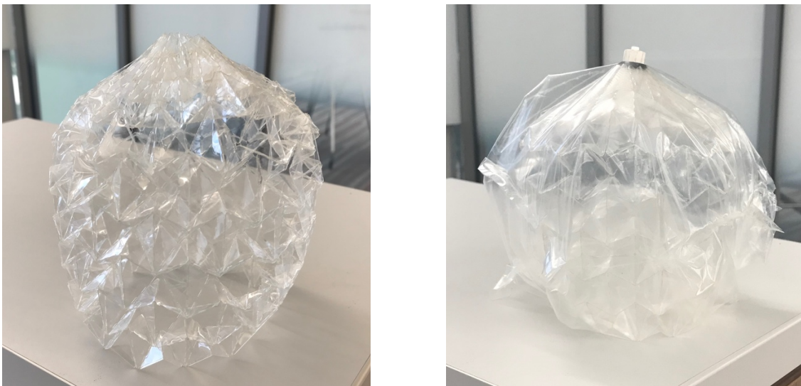
Figure 22. Scaled "magic-ball" gripper design. Skeleton shown left, skeleton with skin shown right.
