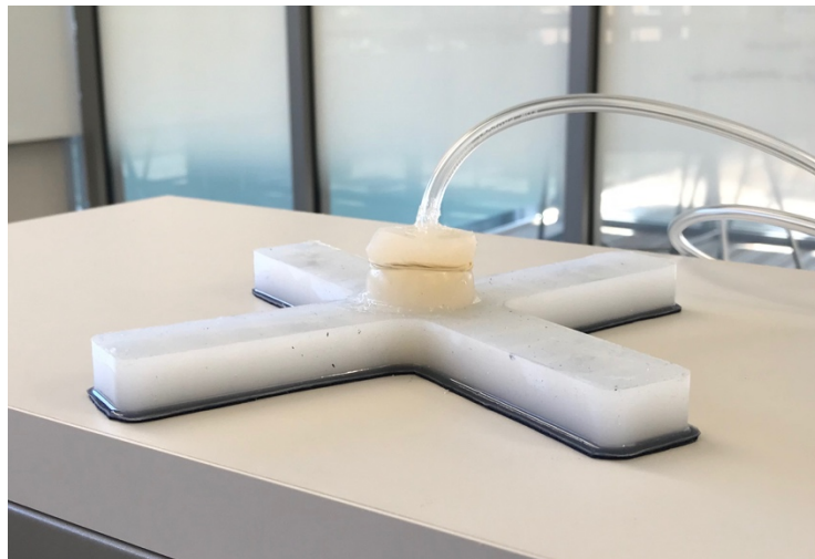
Figure 39. Fabricated PneuNets design.
