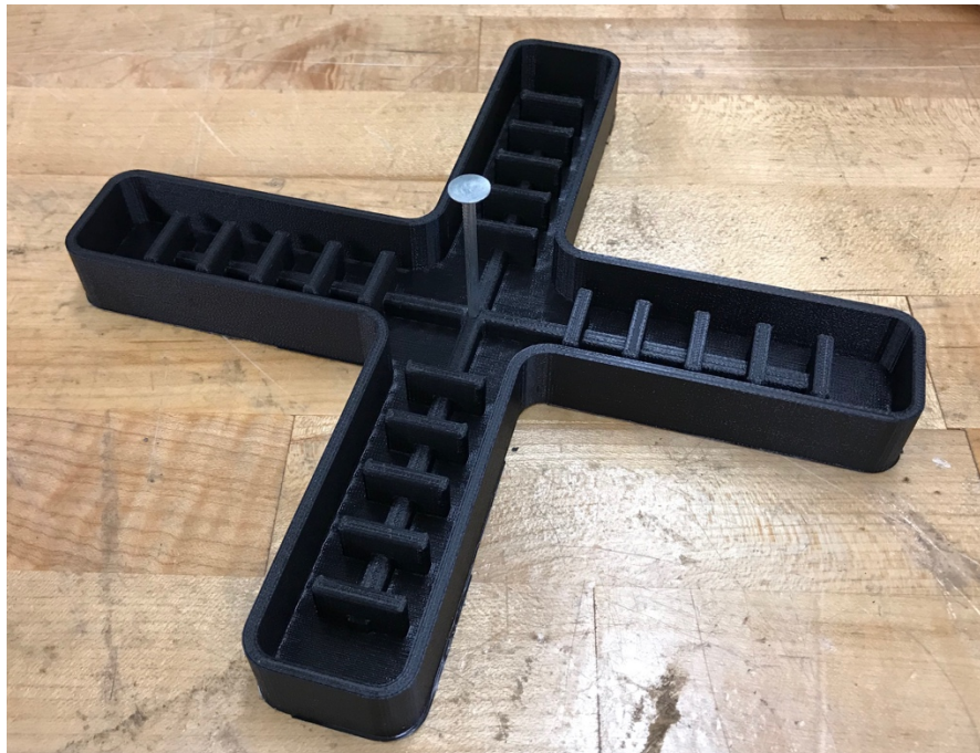
Figure 36. 3D printed PneuNets mold.
