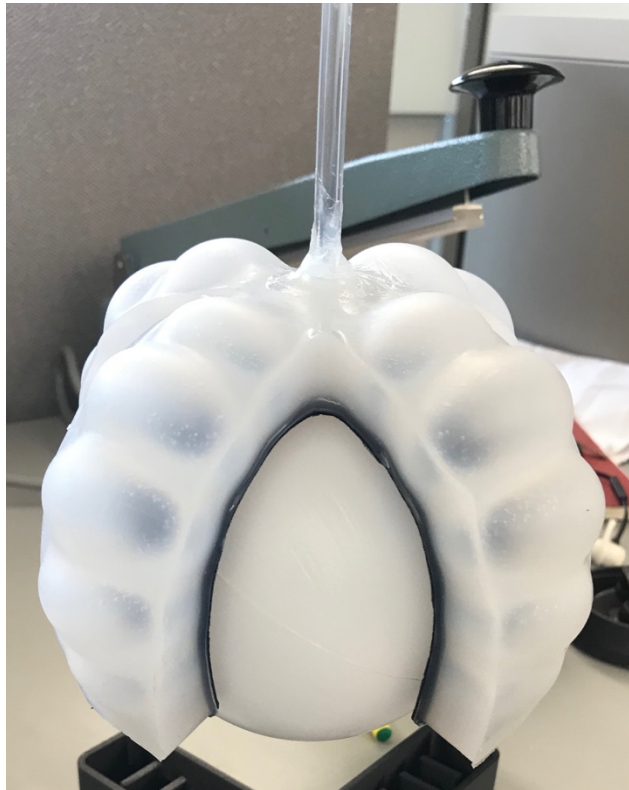
Figure 27. Pneu-Nets design actuated and grasping 3.75" diameter sphere.
