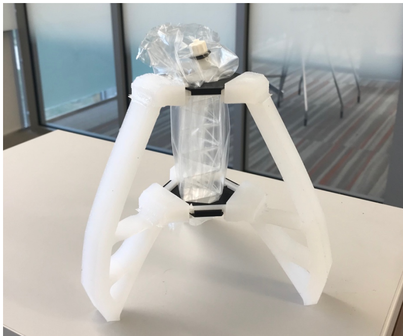
Figure 35. Fully assembled optimal gripper design.
