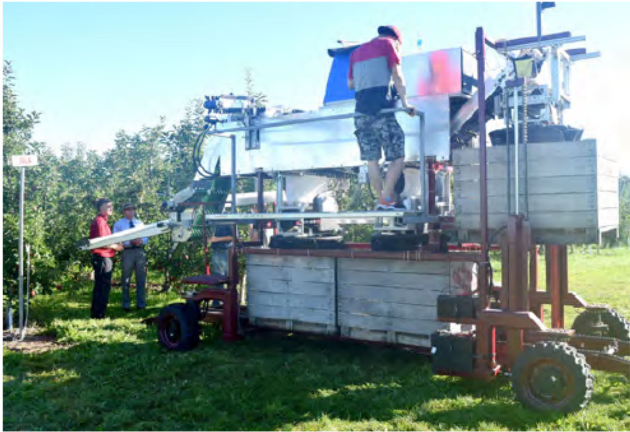
Figure 4. Apple harvesting and infield sorting machine designed by Lu et al. [25].
