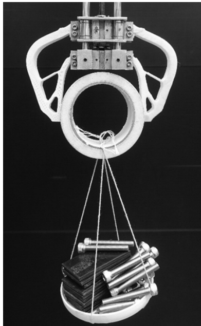
Figure 10. Optimally designed two-finger gripper holding a weighted cylinder [35].
