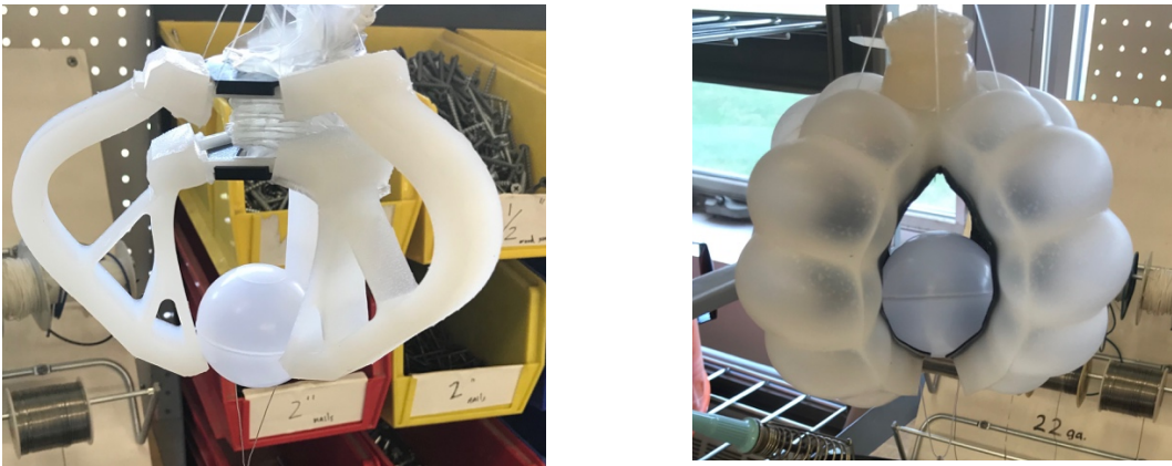
Figure 46. Grasping scheme for the optimal gripper shown left, with caging scheme of the PneuNets design shown right.
