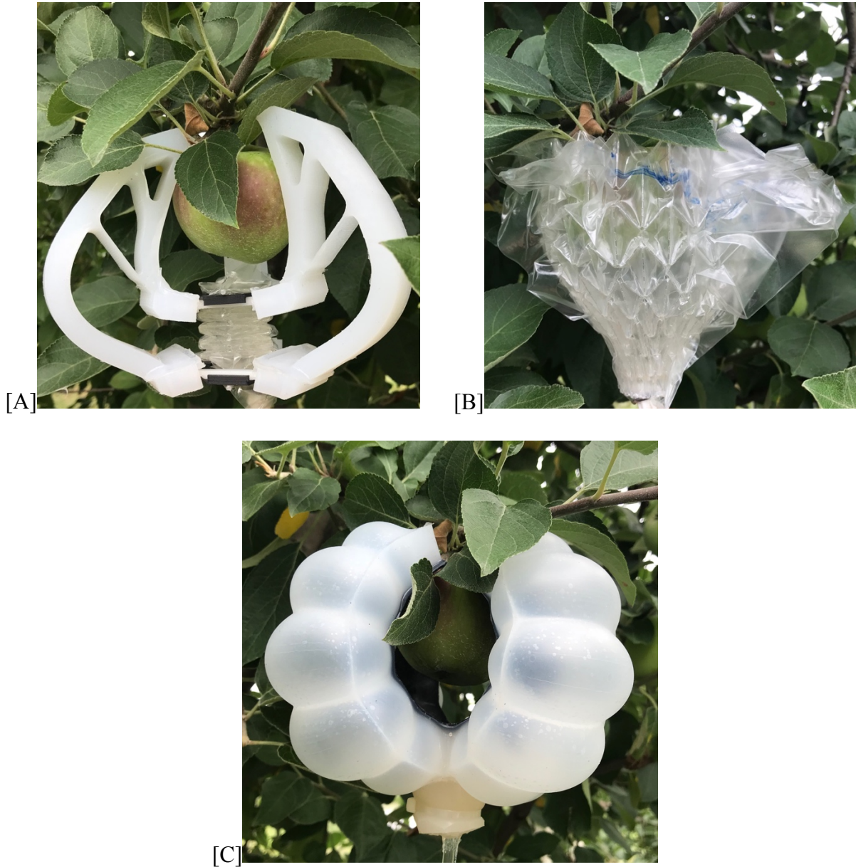
Figure 54. End effectors grasping isolated apples from below.
