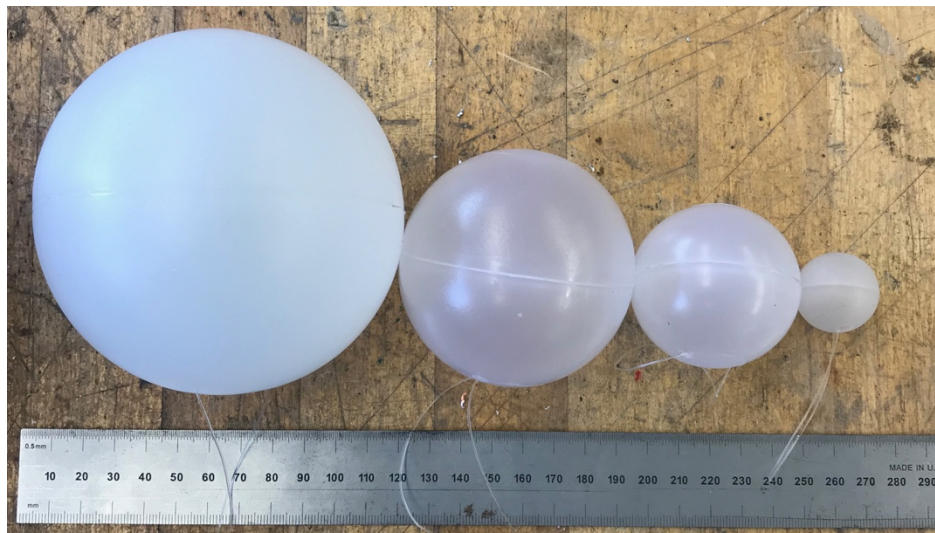
Figure 44. Polypropylene spheres 100, 70, 50 and 25mm diameter with attached monofilament tethers.
