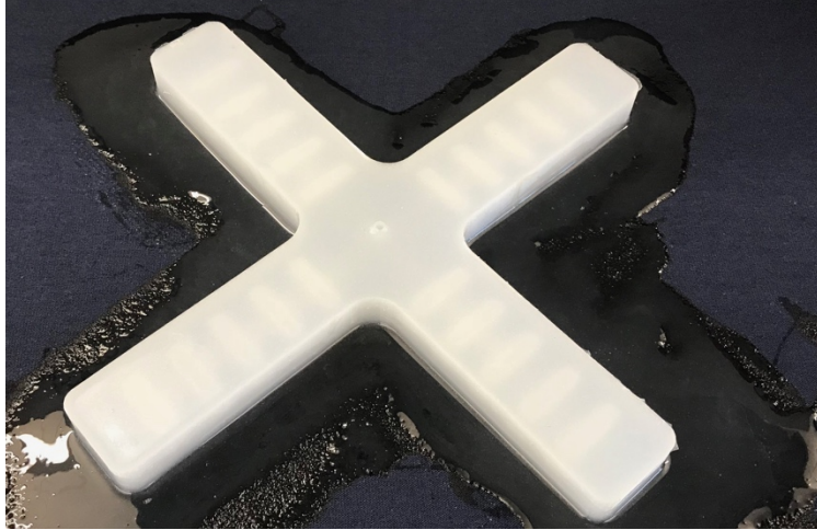
Figure 38. PneuNets top cast curing to cotton layer.
