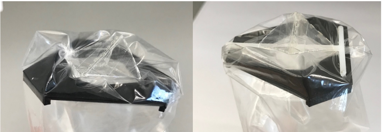
Figure 34. Exposed skeleton after insertion through wafer shown on the left. On the right, the T-shaped pin inserted through the skeleton.
