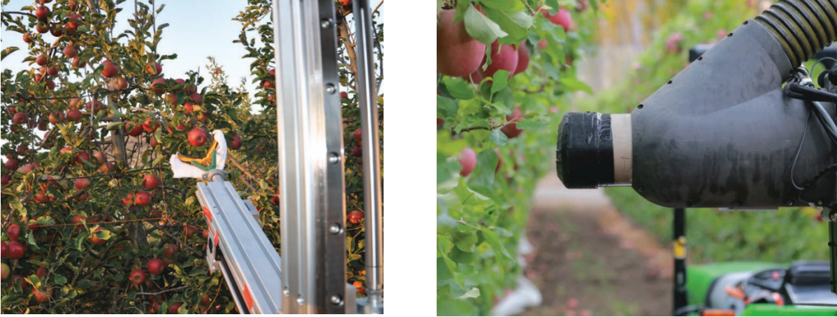
Figure 6. On the Left FFRobotics End Effector harvesting system and on the right is the vacuum harvesting system from Abundant Robotics [28].
