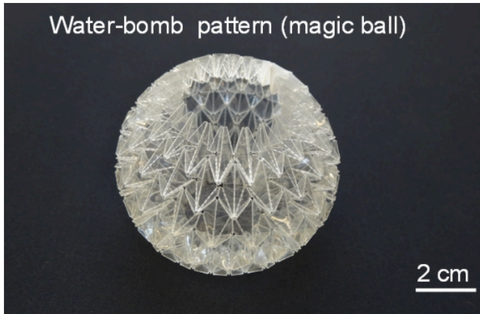
Figure 19. Water-bomb skeleton fold from Li et al [34].
