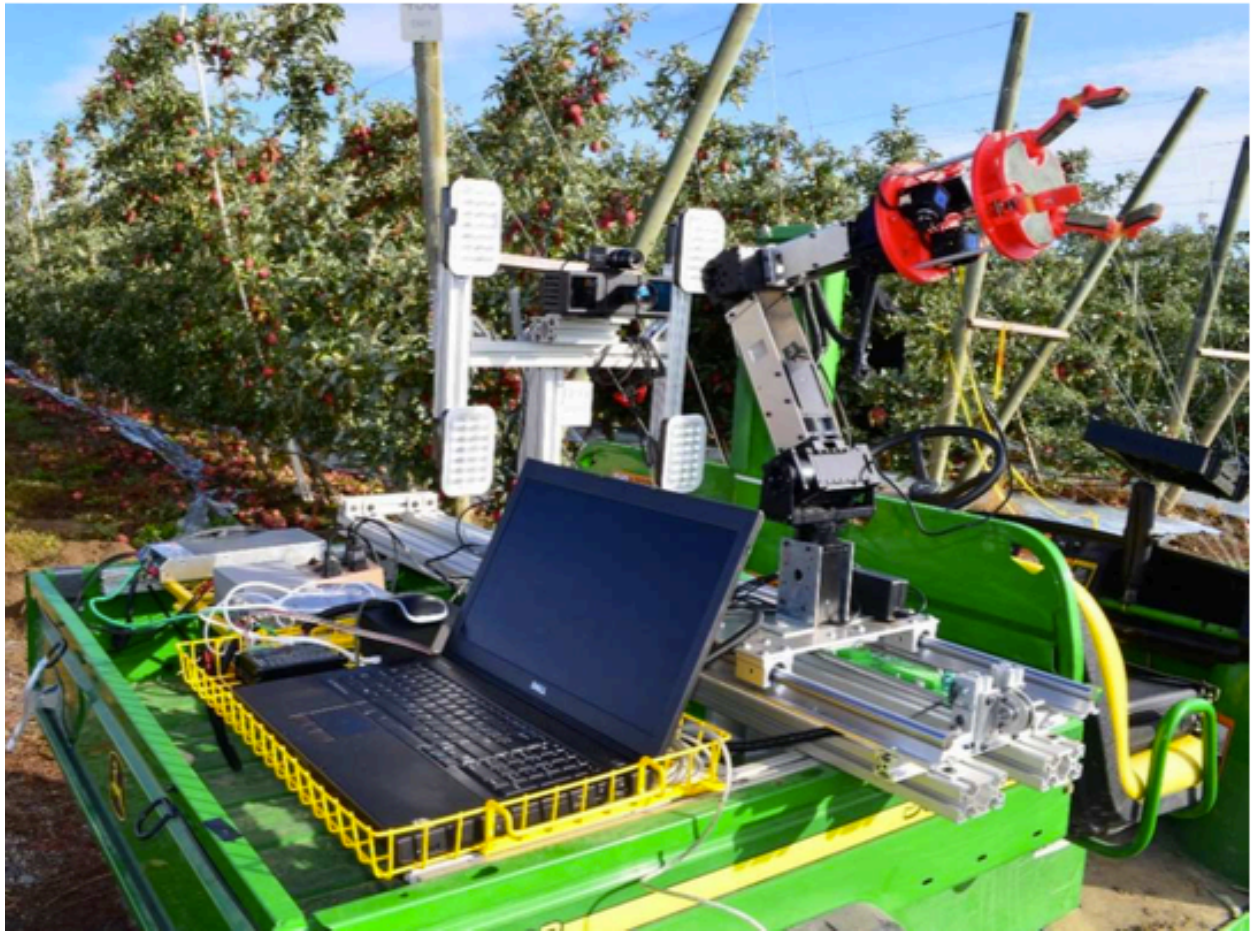
Figure 5. End effector and harvesting platform [27].
