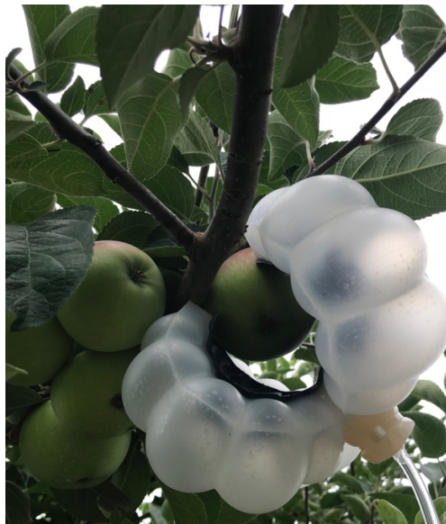
Figure 55. End effectors grasping apples in cluster configuration.
