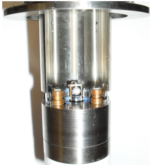
Figure 3.7: STM scanhead, that contains the STM tip and the sample (sample is not placed on the three outer piezo tube in this picture), and will be pushed down into the blue dewar displayed in Figure 3.6. The four piezo tubes of the Besocke design are visible. The STM tip is glued on a Si chip and is positioned on the inner piezo tube in the middle. The magnetic manipulator, displayed in Figure 3.6, will gently place the sample on top of the outer three piezo tubes.
