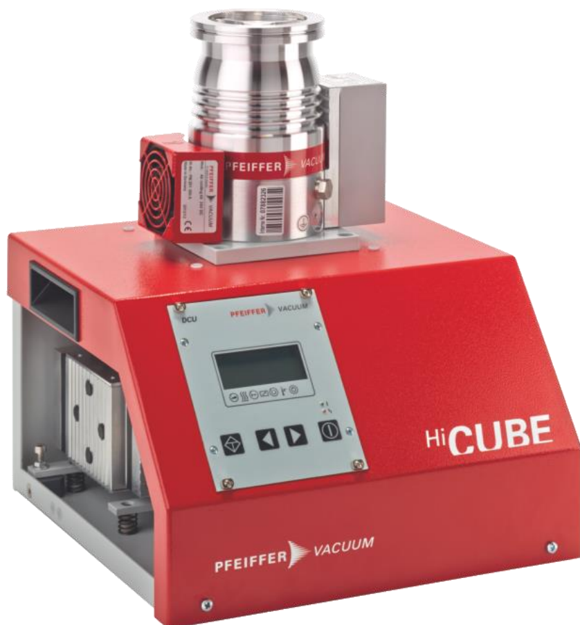
Figure F.3. Pfeiffer Vacuum HiCube 80 Eco pumping station. The bottom houses the control unit and rough pump, and the silver cylinder on top is the turbomolecular pump. A hose is attached at the top of the turbopump and connected directly to the cryostat. Image reproduced from ref. 3 .
