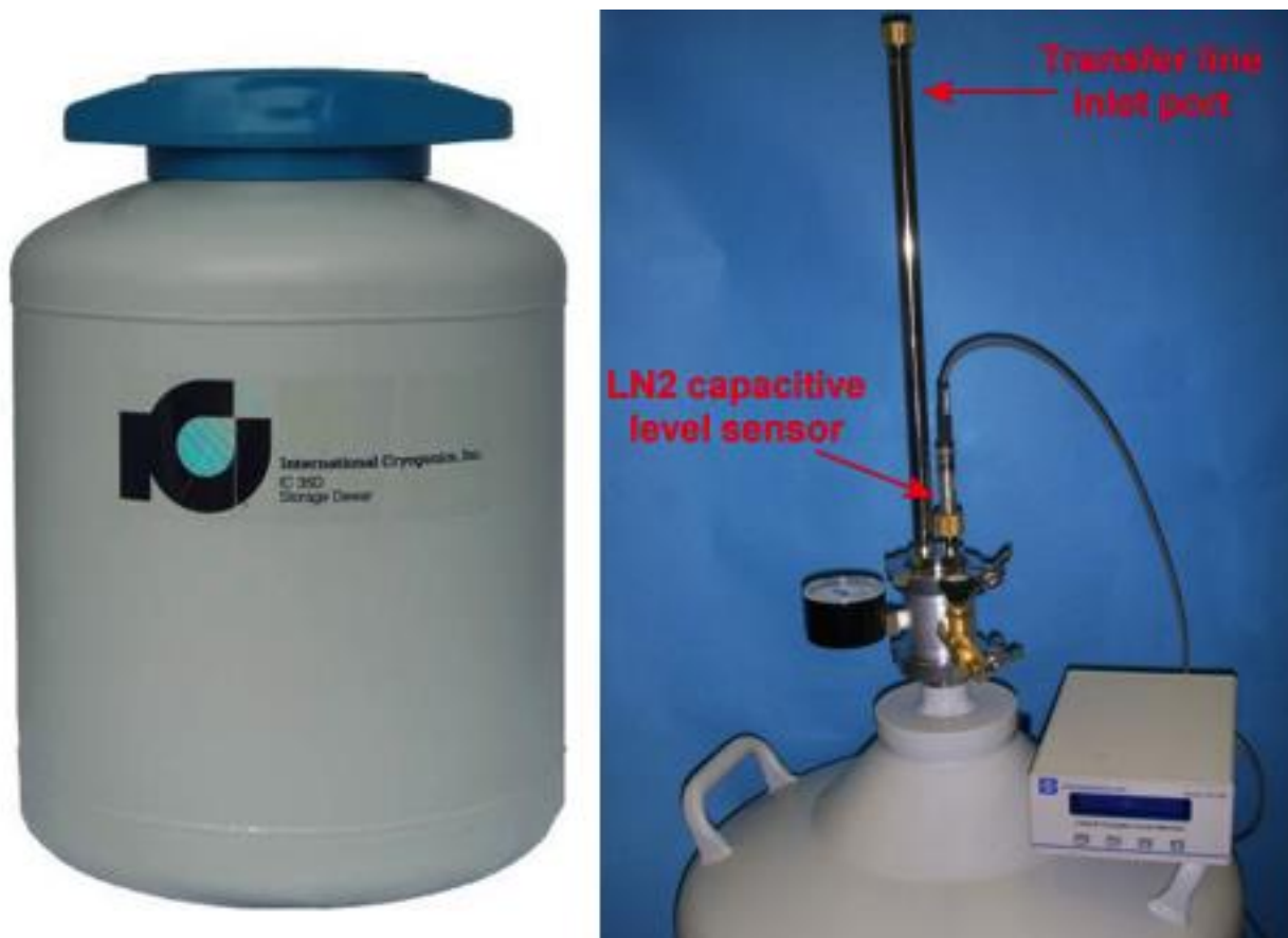
Figure F.4. (Left) International Cryogenics, Inc. 35 L liquid nitrogen storage Dewar utilized in these experiments. Image reproduced from ref. 4 . (Right) Attachments for the storage Dewar, including flanges, pressure gauge, and transfer line inlet port. The liquid nitrogen capacitive level sensor shown above is not included in our set-up. Image reproduced from ref. 1 .
