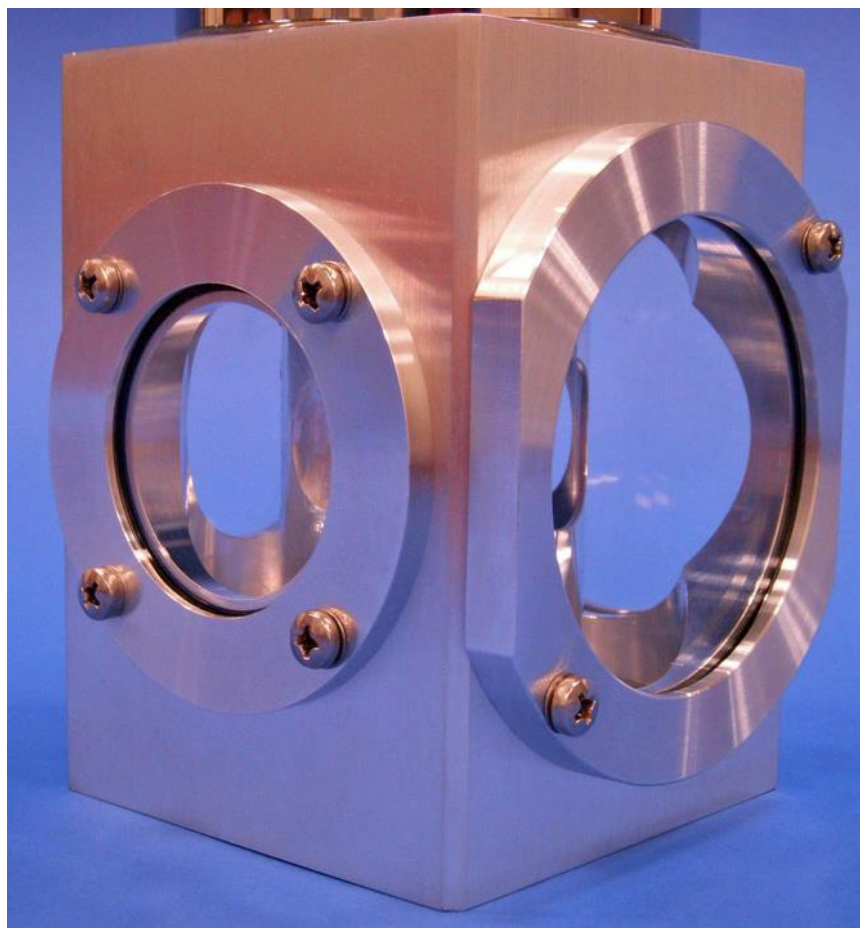
Figure F.2. Blow-up of the bottom-most portion of the optical Dewar from Janis Research. Each of the outer- and inner-jacket have four optical windows, allowing for collinear of 90^\circ experiments to be performed in this one cryostat. Image reproduced from ref. 1 .
