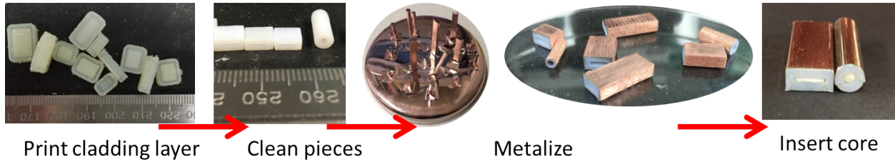
Figure 3.2: Visualization of the general fabrication process for the waveguiding structures made in this work.
