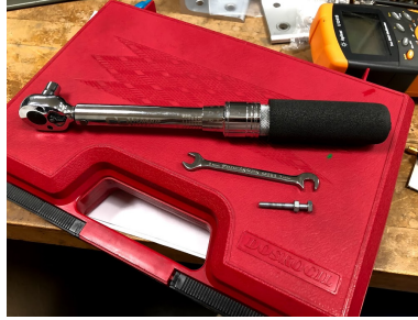
Figure B.4: Adjustable socket torque wrench setup for use with the X-Band flange bolts with additional holding wrench and example bolt.
