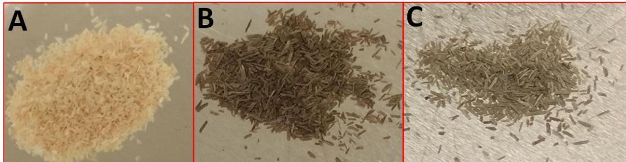
Figure 5.4. Images of raw birch biomass (A), and after pretreatment at 220 °C in ethanol with no catalyst (B), and with Co/C catalyst (C).
