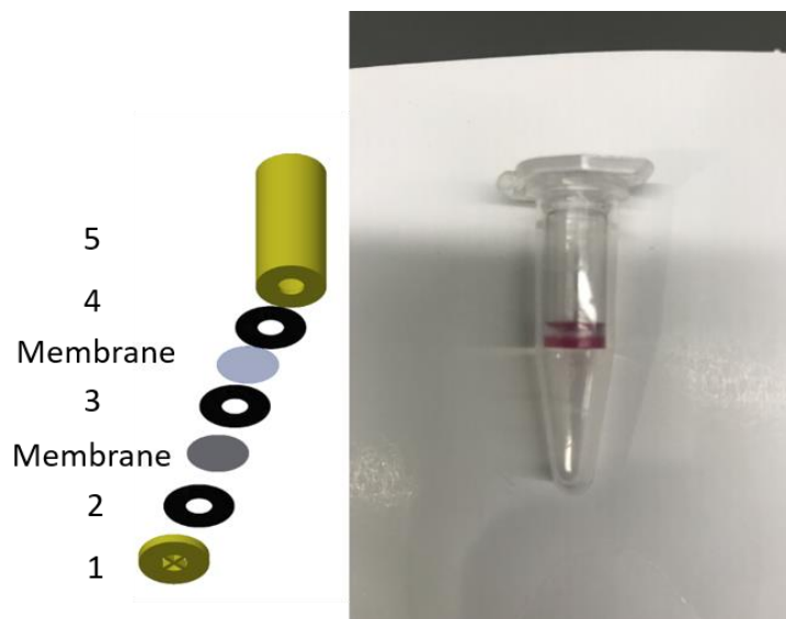
Figure 3.5 3D-printed Centrifuge-Enabled Ultrafiltration Device Left: A CAD drawn schematic diagram showing the individual parts of the 3D-printed device, including both membranes. The numbers refer to the order in which each part was printed. Right: A photograph of the device ready to be used by being placed into a centrifuge tube.
