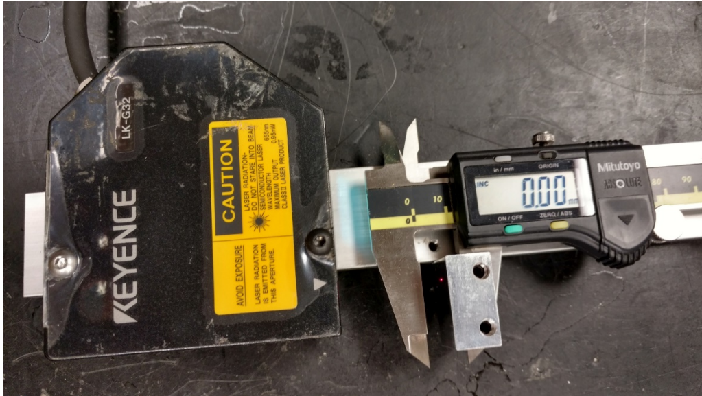
Figure 15: Laser position sensor calibration fixture used to verify sensitivity and linearity.
