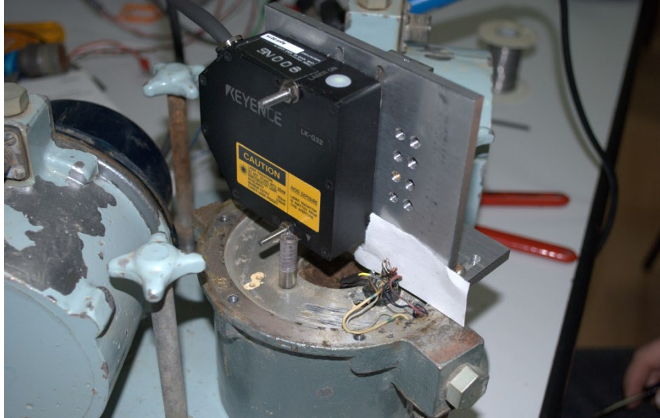
Figure 37: S1-P Seismometer, as used in Kazakhstan, with custom laser mounting bracket.
