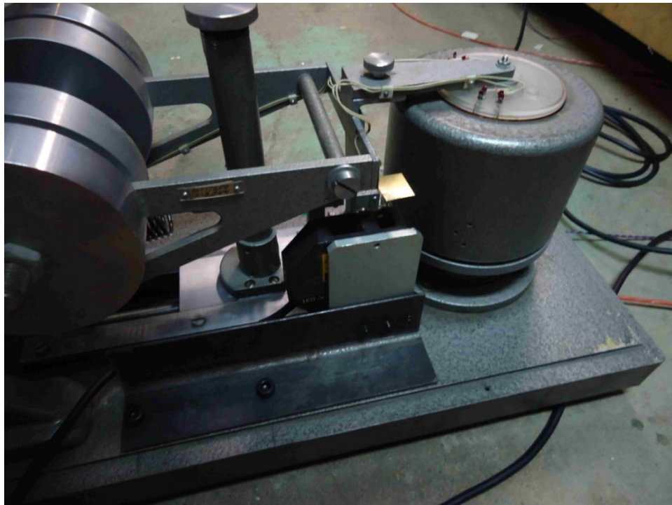
Figure 36: The LK-31 laser mounted on an SKM-V seismometer. The laser measures displacement via the brass reflector that is permanently attached to the pendulum arm.
