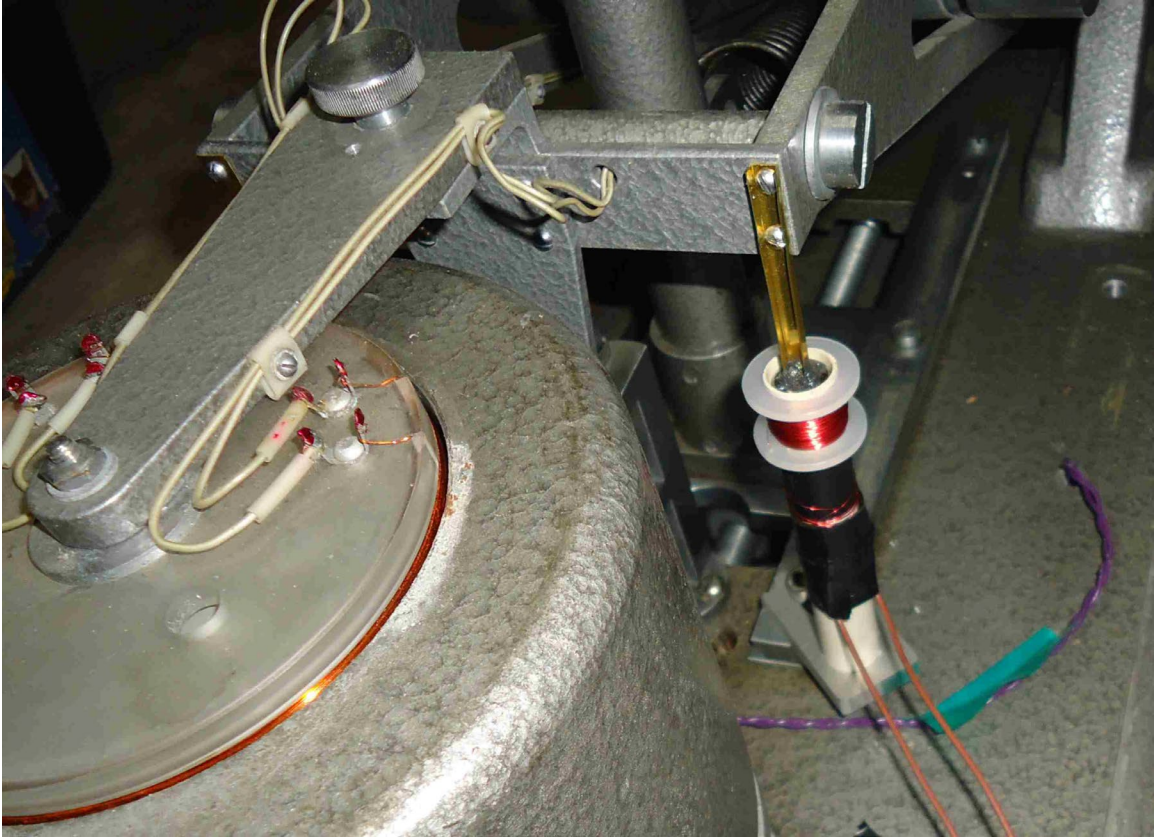
Figure 12: Excitation coil mounted on the base of a Russian SKM seismometer. The armature-mounted brass fixture contains a small neodymium magnet that enables us to apply a sinusoidal electromotive force to the pendulum with a signal generator.
