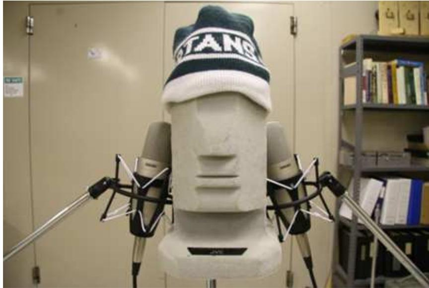
Figure 2.3: During playback of the phonetically-balanced sentences through a loudspeaker (not shown) in Room 10B, two cardioid microphones were located on opposite sides of a plastic “head.” The plastic head simulated head diffraction. Recordings from the cardioid microphones were played over headphones to listeners in Experiment 3.
