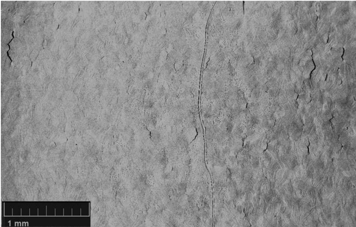
Figure 5.31 Low-magnification SE SEM micrograph of a RT deformed TNTZ-0.3O sample. Some boundary cracks were observed throughout the gage section. The tensile axis was horizontal.
