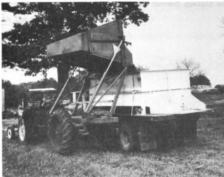
Figure 8. 3.2 Metric Ton Capacity, High Lift Bulk Handling System to Replace Conventional Vineyard Trailer - 1973.
