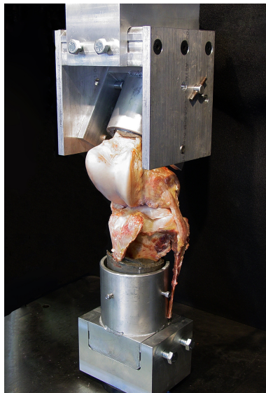
Figure 5.1 Cadaver stifle loaded in the custom aluminum testing fixture at 150^{\circ} stifle angle.
