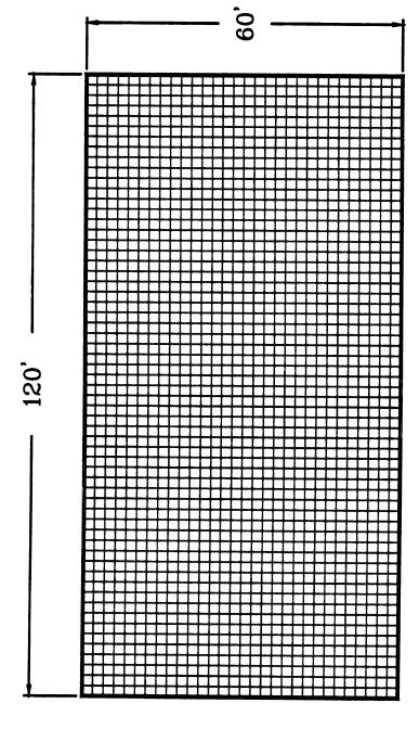
Horizontal and vertical grid lines are 2' on center.
