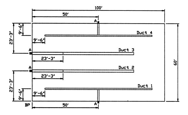
Figure 14. Sample aeration system plan displayed and printed for user of aeration system design program.
