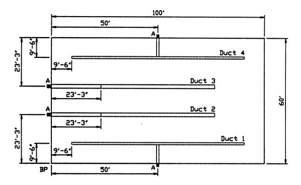
Figure 5. Sample customized plan view drawing of an aeration system, representing a design drawing to be provided to a client.
