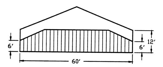
Vertical grid lines in grain area are 2' on center.
