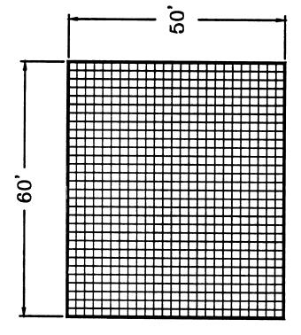
Horizontal and vertical grid lines are 2' on center.
