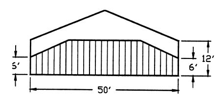
Vertical grid lines in grain area are 2' on center.
