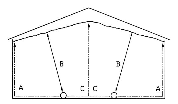
A -- air path from duct to grain surface along outside wall
