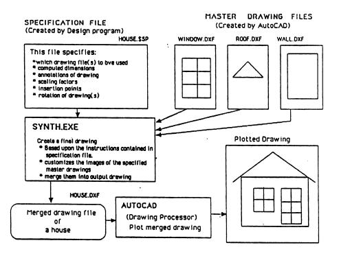
Figure 7. Functional description of Synthesis and AutoCAD usage to produce a parameterized design drawing.
