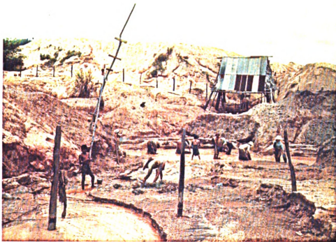
Exhibit 9 - 'Panning' the ores in the valley or left-over areas in the gravelpump or opencast mines. It is normally done by women and children.
