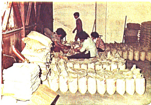
Exhibit 10 - In the dressing shed the ore concentrates are packed in small bags before they are sent to smelters.
