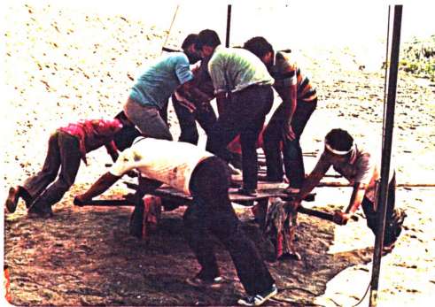
Exhibit 1 - Prospecting the tin ore by using a boring tool. The results of this test-boring will determine the exact location of the ores to be mined.
