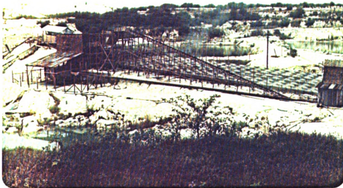
Exhibit 6 - A closer view of a 'palong' which is about 30 feet wide and 130 feet long. The 'palong' is used in gravelpump as well as in other opencast mines.
