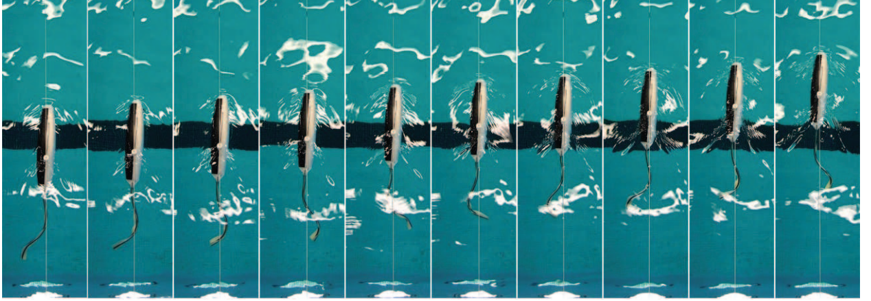
Figure 5.2: High-speed images of the submersible with the flexible tail acquired over a period of 1 sec, soon after it started from rest in the MSU swimming pool. The average speed of the submersible in these images was \approx 0.4 \text{ BL/s} , less than the maximum speed of \approx 1.15 \text{ BL/s} . Note the large deflections of the tail which occur during acceleration.
