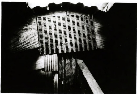
Figure 4.2. Failure at the Wood-Metal Fastener Connection, Barn J.
