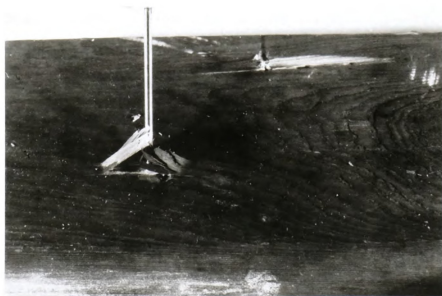
Figure 4.5. Pick test. Brash break indicates presence of decay.
