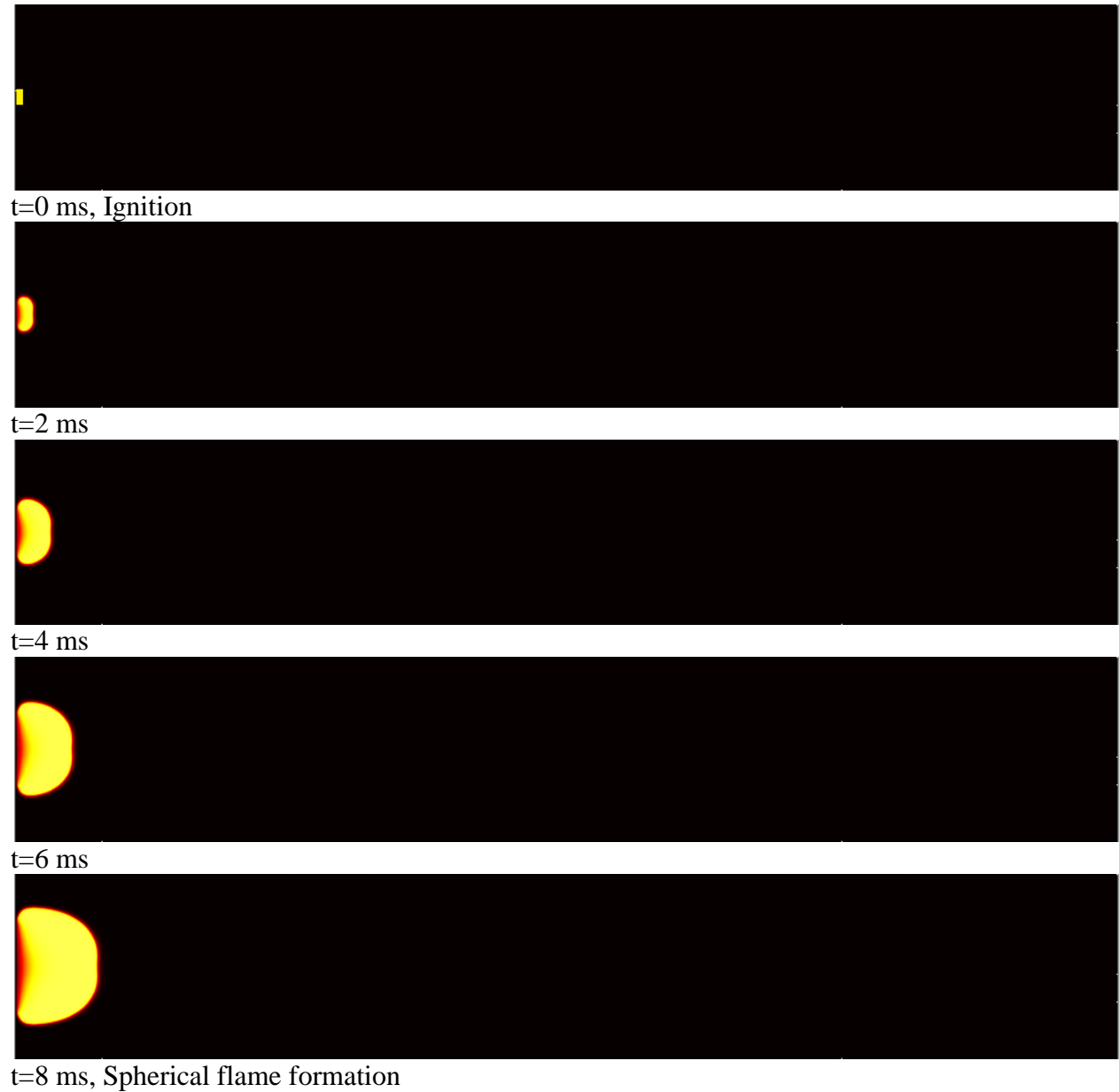
Figure 5.3 – Flame propagation along the combustion tube, showing the evolution of the flame structure from ignition to finger flame formation.
