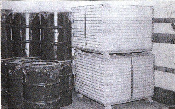
Figure 2. Allied's Aftermarket Division was one of the first to adopt a plastic bulk-bag for a liquid product. 225 gallons of "Plastisol" adhesive, which is the viscosity of caramel (45,000 centipoise), is packaged in a multiple-component "bag in a box," replacing 55-gallon steel drums. The adhesive is shipped to Allied to be used in the manufacture of air filters for vehicles. The package has 4 components (listed from outside in):
