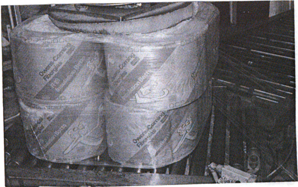
Figure 7. Owens-Corning Fiberglas makes rolls of insulation which have always been shipped break-bulk. Their innovative package is a unitization method which results in a multiple-roll distribution package which can be handled either mechanically or by hand. The rolls of insulation are stretch-wrapped together, in a footprint of 4, two or four high. (Each roll is already "packaged" in a paper wrapper which is applied at the time of rolling; the ends are open.) This is the only case study in this research which documents a change in the number of products in a package and goes from a manual to a mostly mechanical handling system. It is included because of its unique departure from conventional pallet-load unitization methods.
