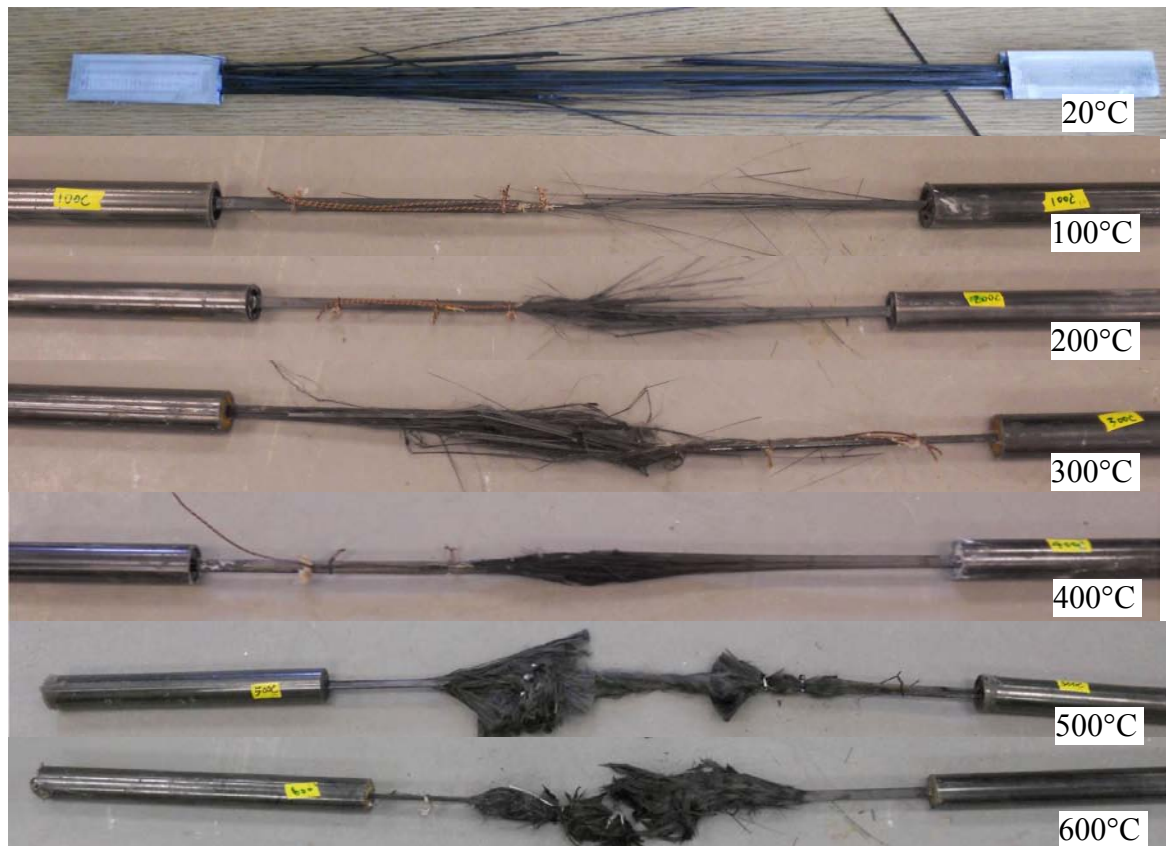
Figure 3.10 Failure modes of CFRP strips at various temperatures
