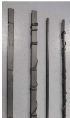
(b) Wires on FRPs
