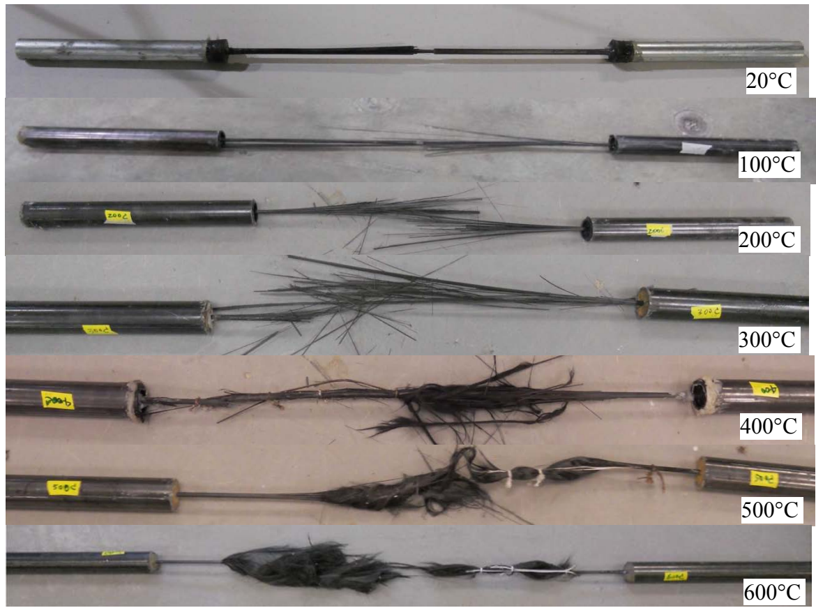
Figure 3.11 Failure modes of CFRP rods at various temperatures
