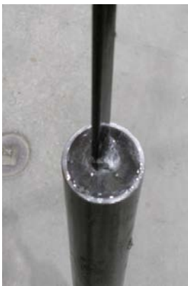
(a) Epoxy filling
