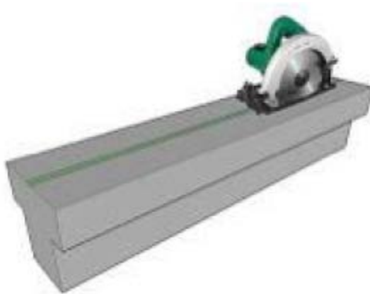
(a) Cut grooves on concrete cover
