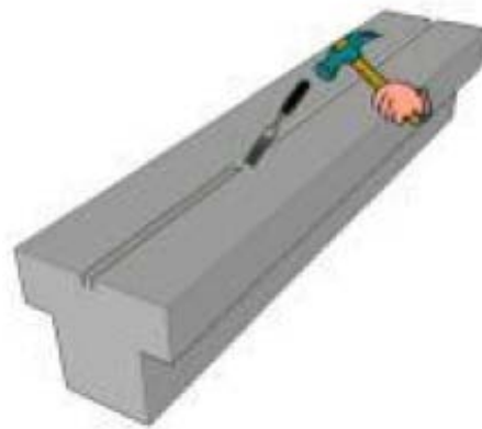
(b) Chisel remaining concrete in groove
