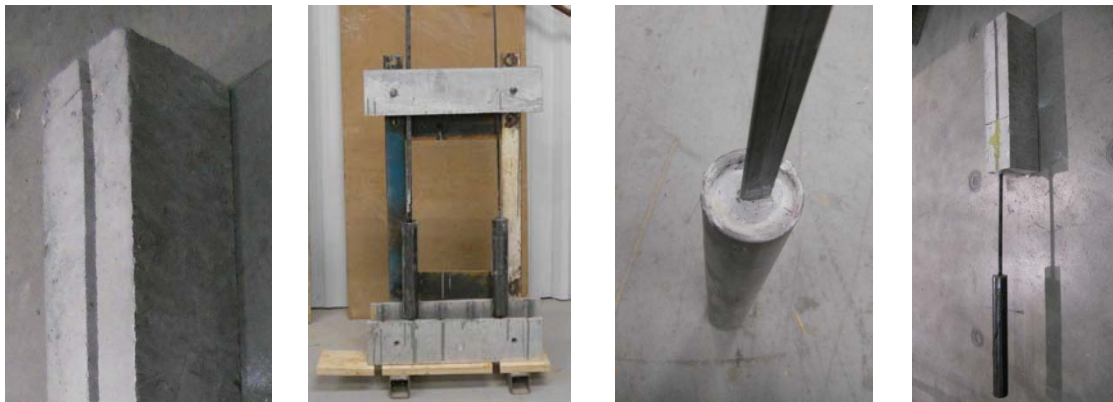
(a) Concrete block (b) Steel frame for anchor (c) Filling cement (d) Test specimen
