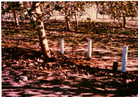
Figure 3.1. Field installed minirhizotrons at 30 cm intervals in one of the Eugenei well watered treatment trees.
