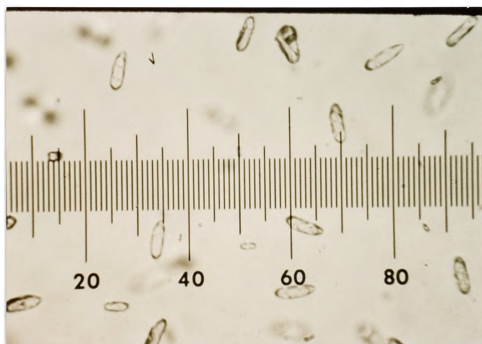
Figure 5-26. COM Crystals of Figure 5-25 After Growth in 8 mg/l Polyglutamate at \sigma = 3.71 and T = 37^\circ\text{C} .
