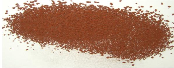
**Figure 2.**”For the interpretation of the references to color in this and all other figures, the reader is referred to the electronic version of the thesis.” Granular, Iron Foam Substrate Coated with Nano Iron. (Photo Courtesy of Dr. Steven Safferman).
