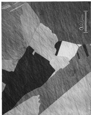
Fig. 39. The metallograph of pure Ni, compressed at 850°C with 2 \times 10^{-5} \text{ s}^{-1} .
