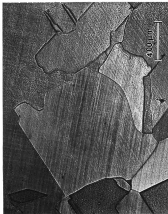
Fig. 40. The metallograph of pure Ni, compressed at 1000°C with 2 \times 10^{-4} \text{ s}^{-1} .
