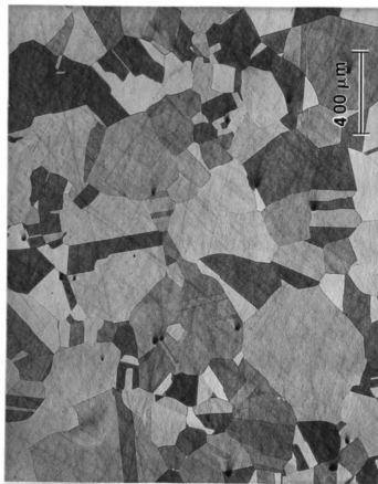
Fig. 6. The metallograph of pure Ni annealed at 1000°C for 30 min.
