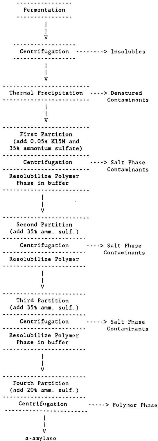
Figure 3.11. The downstream purification of  $\alpha$ -amylase.
