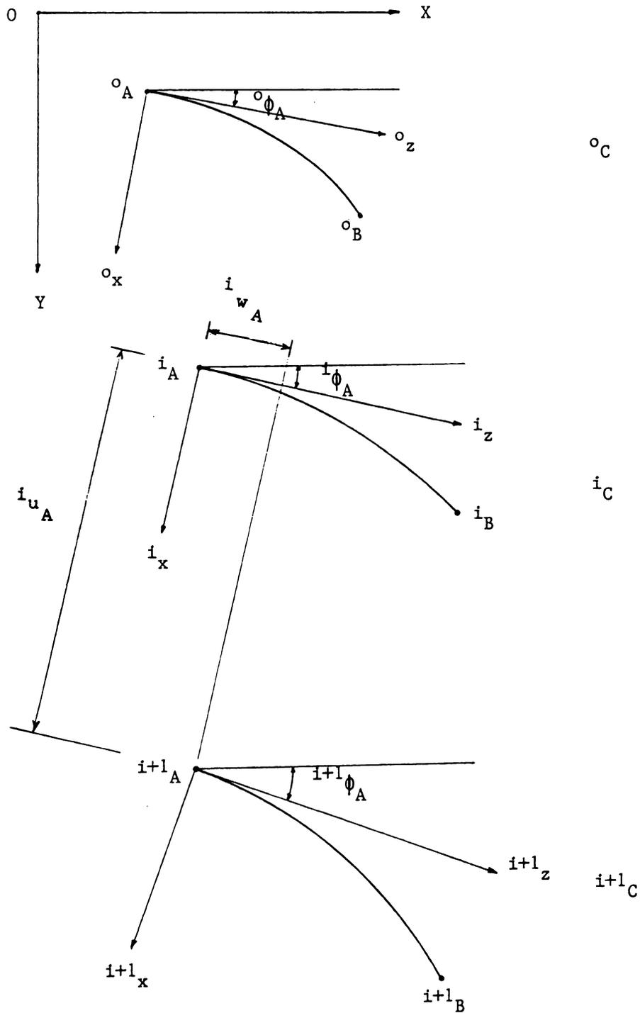
Figure A-1 : CONFIGURATION OF A TWO DIMENSIONAL CURVED BEAM ELEMENT AT SUCCESSIVE LOAD INCREMENTS IN UPDATED LAGRANGE FORMULATION
