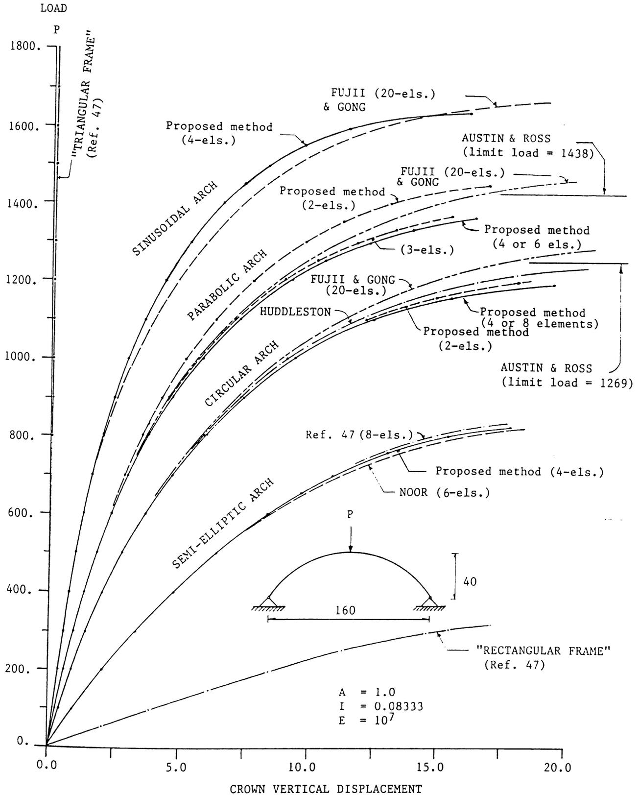
FIGURE 4-15 : SINUSOIDAL, PARABOLIC, CIRCULAR, SEMI-ELLIPTIC ARCHES, TRIANGULAR FRAME, AND RECTANGULAR FRAME SUBJECTED TO A CONCENTRATED LOAD AT THEIR CROWNS
