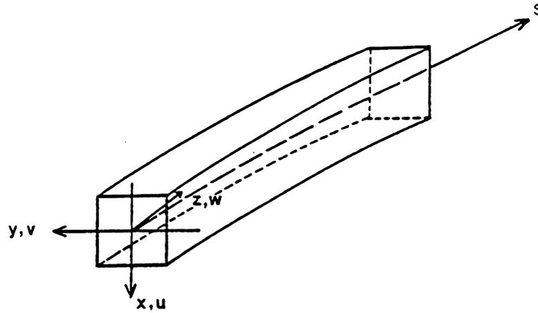
Figure 2-1 : BEAM ELEMENT (Curved In The  $x$ - $z$  Plane)
