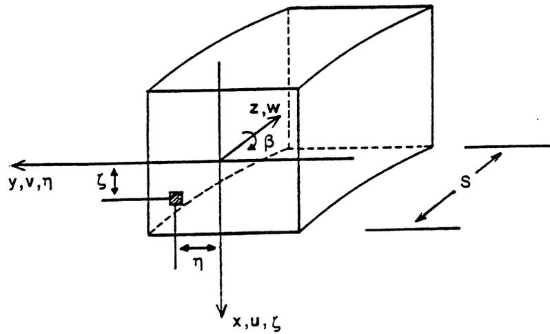
Figure 2-2 : CROSS-SECTION OF PRISMATIC MEMBER
