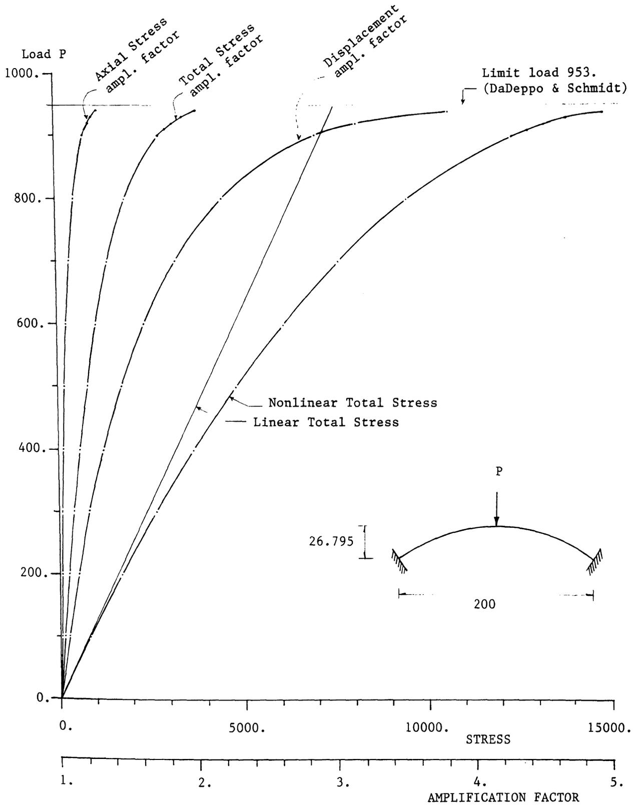
FIGURE 4-19 : STRESSES AND AMPLIFICATION FACTORS AT THE CROWN
