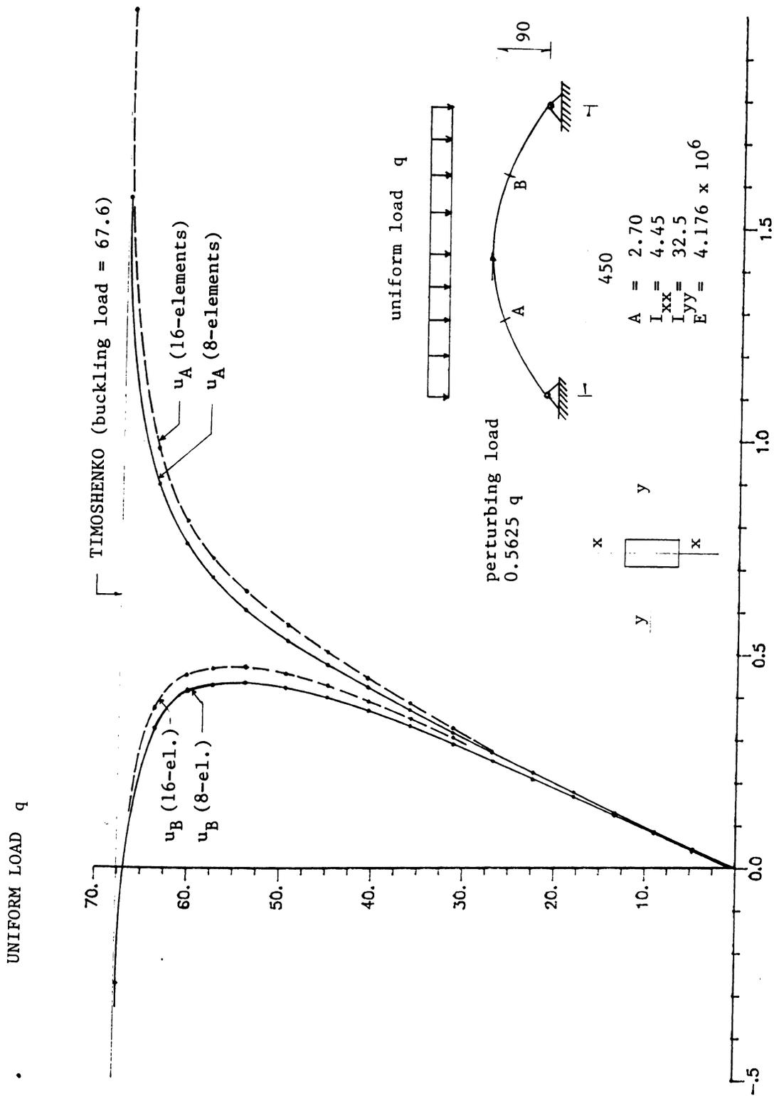
FIGURE 4-5 : A HINGED PARABOLIC ARCH SUBJECTED TO UNIFORM LOAD ON HORIZONTAL PROJECTION (IN-PLANE BEHAVIOR)
