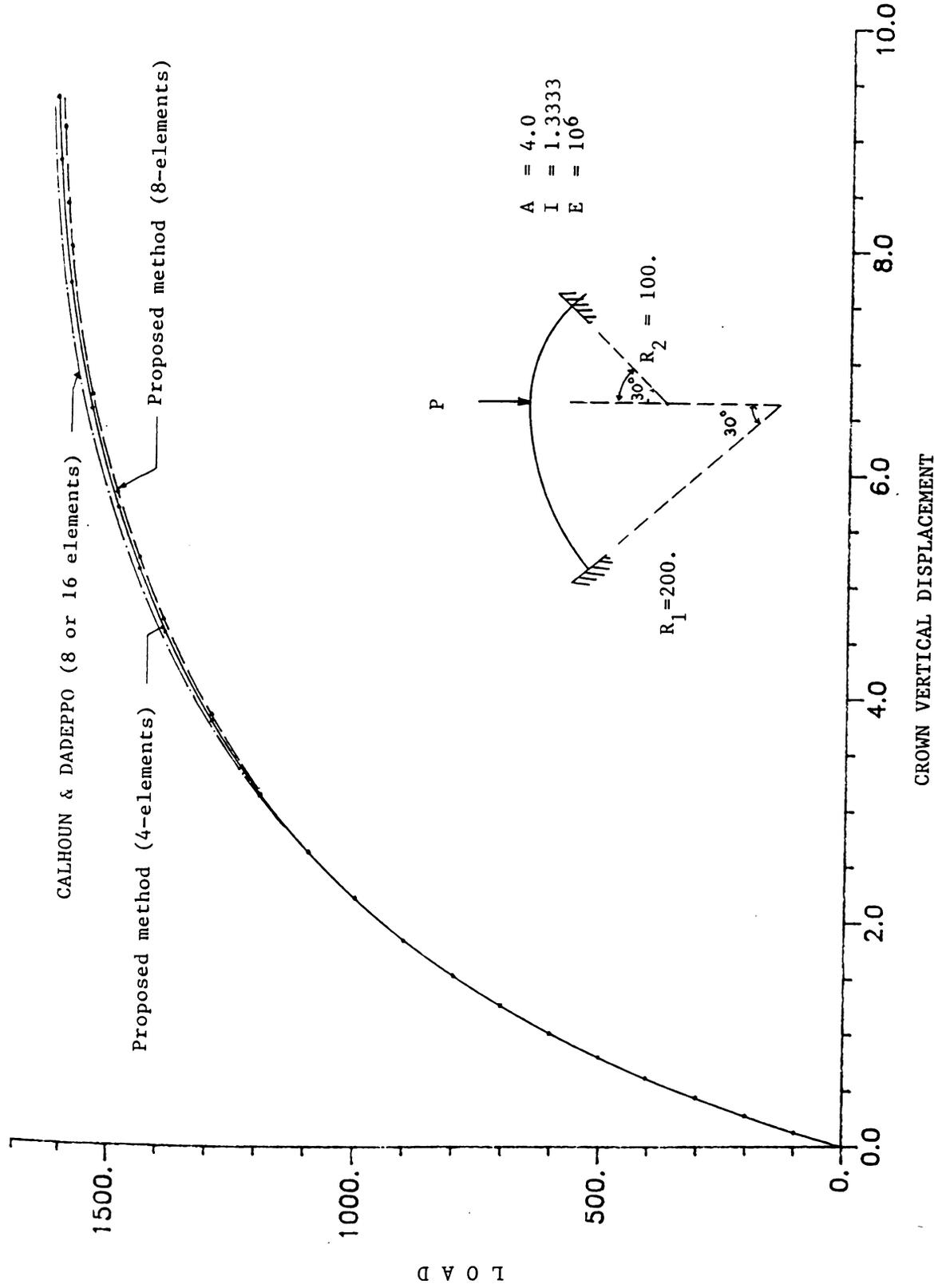
FIGURE 4-11 : A CLAMPED MULTIPLE RADII CIRCULAR ARCH
