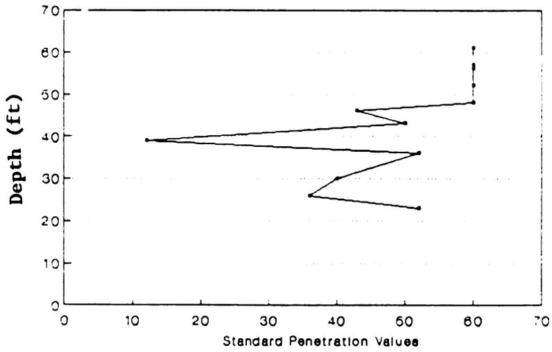
**Figure 34. Results of Standard Penetration Test for a Student Center in Germany**
