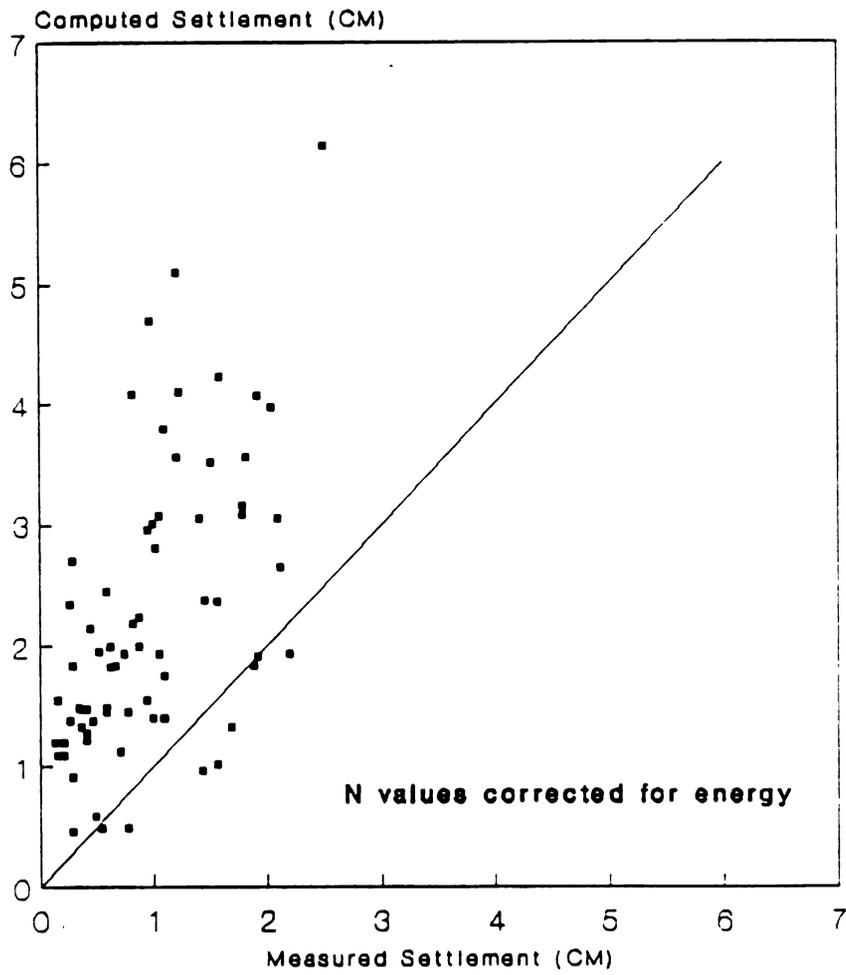
**Figure 28. Comparison Of Measured Settlements With Values Computed By Meyerhof Method**
