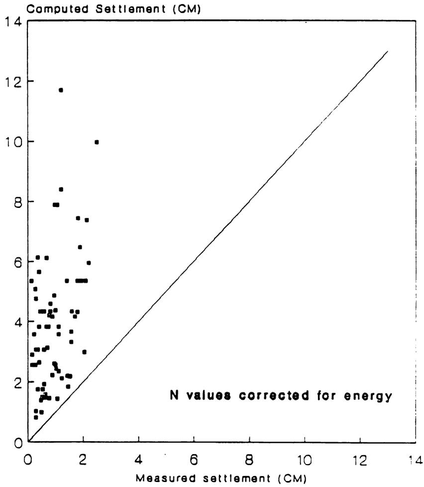
**Figure 31. Comparison Of Measured Settlements With Values Computed By Bazaraa Method**
