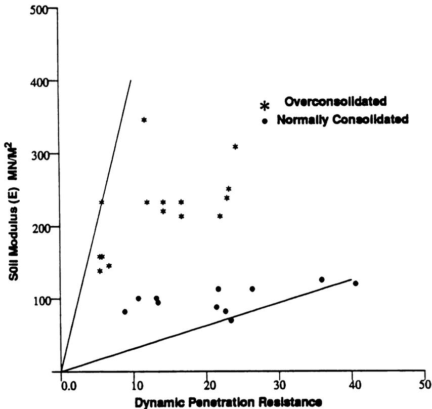
**Figure 4. Relationship between Tangent Modulus and Dynamic Penetration Values for Normally consolidated and Overconsolidated Sands ( After, Clayton et al. 1988)**
