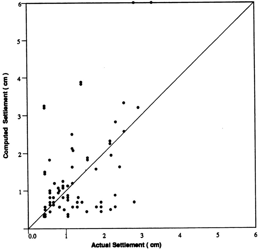
**Figure 9 . Comparison of Measured Settlements with Values Computed by Terzaghi Method (after Jayapalan and Boehm, 1985 )**
