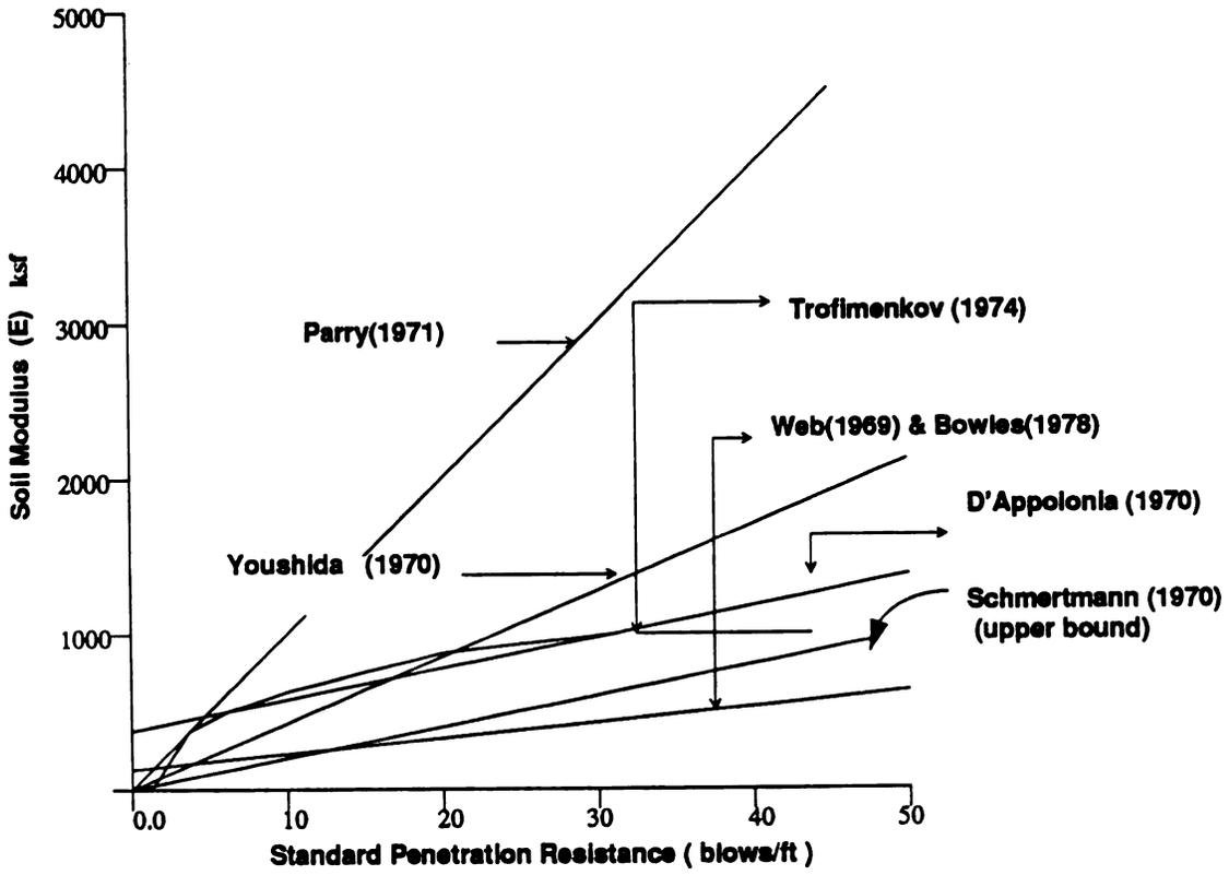
Figure 3 . Relationship between Modulus of Elasticity and Standard Penetration Value for Different Methods
