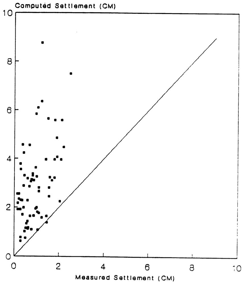
**Figure 26. Comparison Of Measured Settlements With Values Computed By Bazaraa Method**
