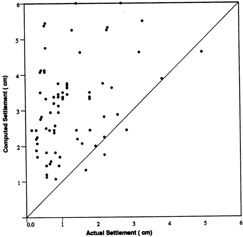
**Figure 5. Comparison Of Measured Settlements with Values Computed by Meyerhof's Method (after, Jayapalan and Boehm, 1986)**
