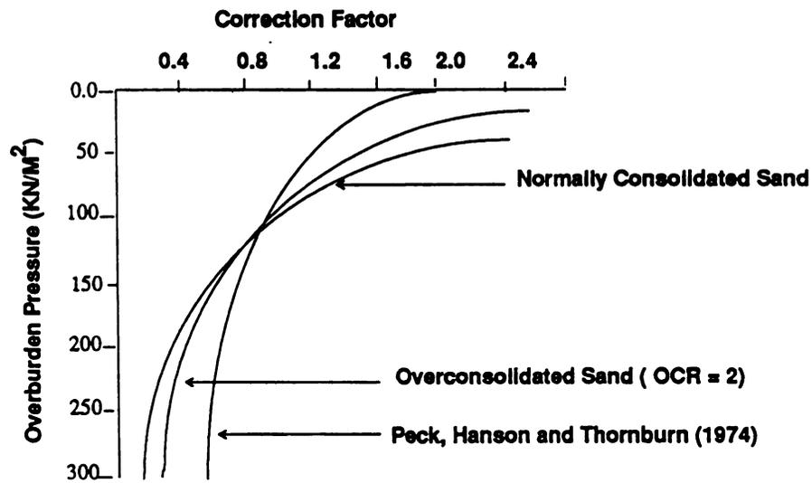
Figure 2. Effect Of Overburden Pressure on Penetration Resistance (after, Hababa (1984)).
