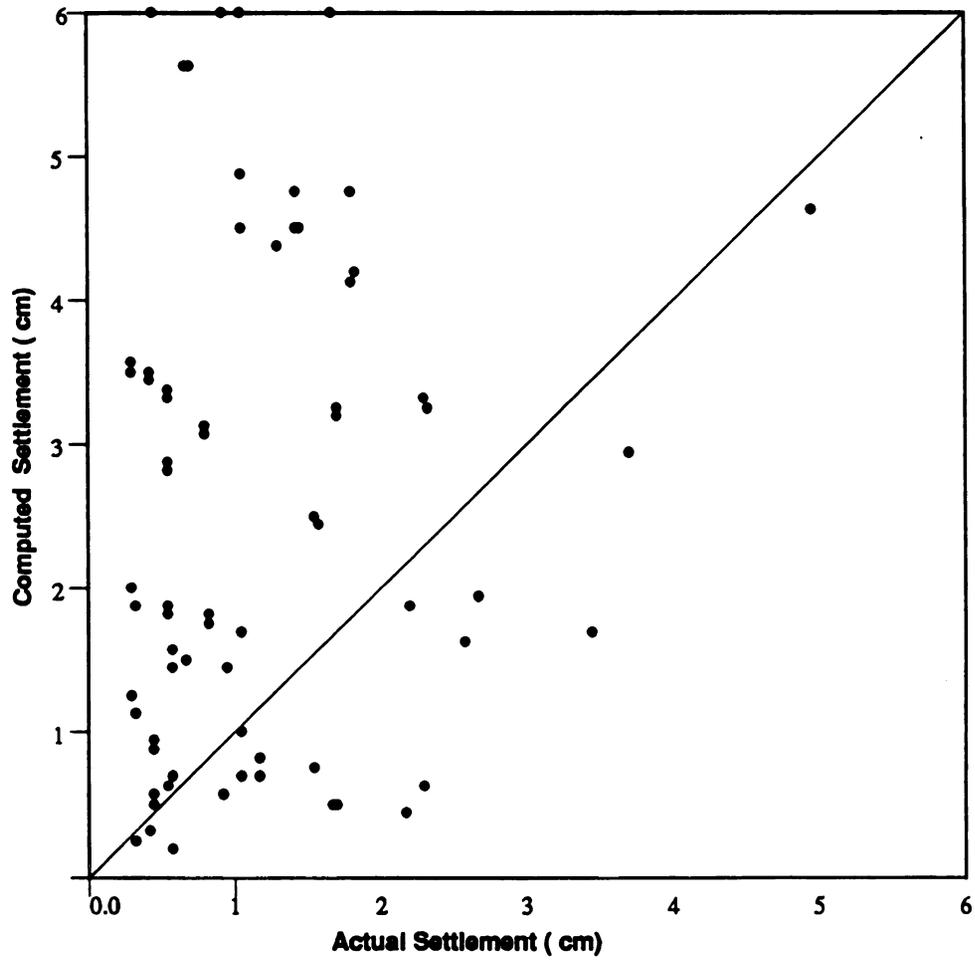
**Figure 6 . Comparison of Measured Settlements with Values Computed by Oweise's Method (after, Jayapalan and Boehm , 1986)**
