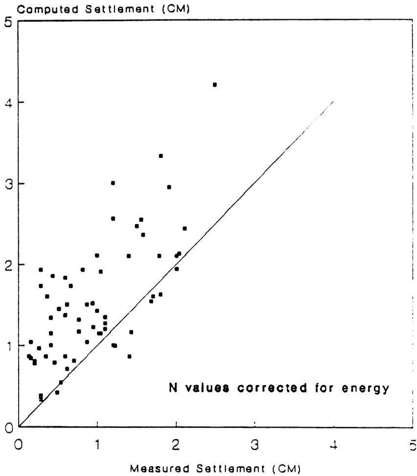
**Figure 27. Comparison Of Measured Settlements With Values Computed By Suggested Method**
