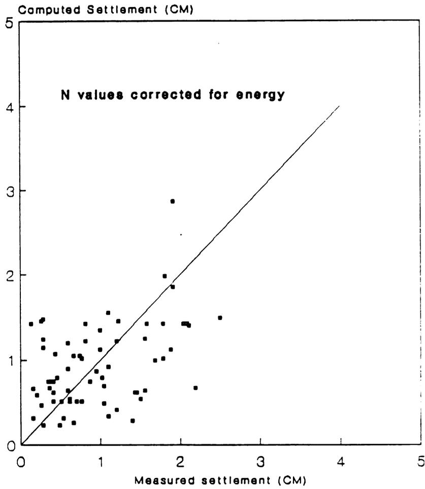
**Figure 29. Comparison Of Measured Settlements With Values Computed By D'Applonia Method**
