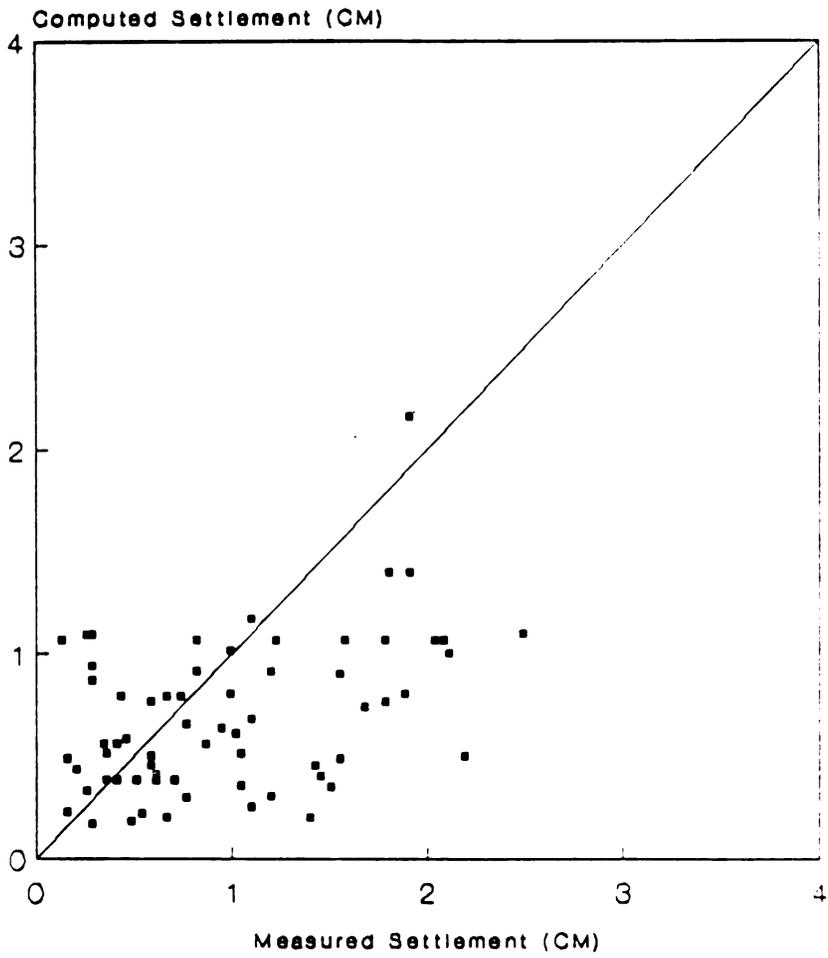
**Figure 24. Comparison Of Measured Settlements With Values Computed By D'Applonia Method**
