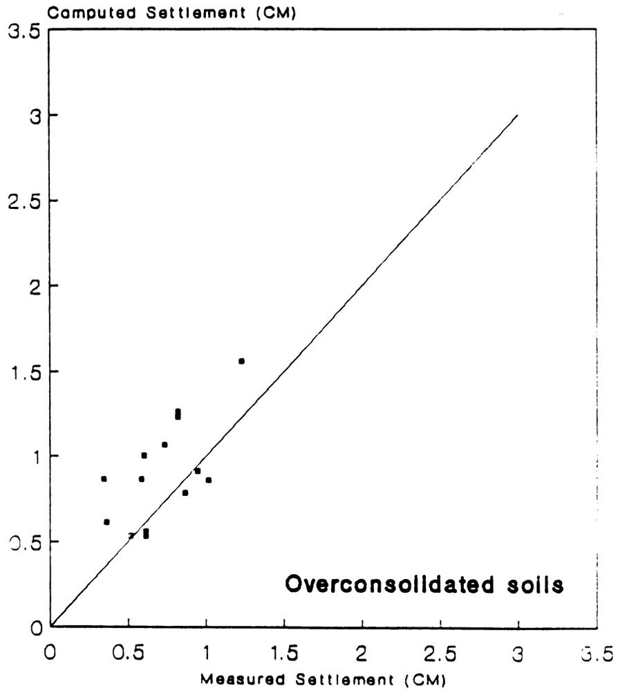
**Figure 13. Comparison Of Measured Settlements With Values Computed By Proposed Method**
