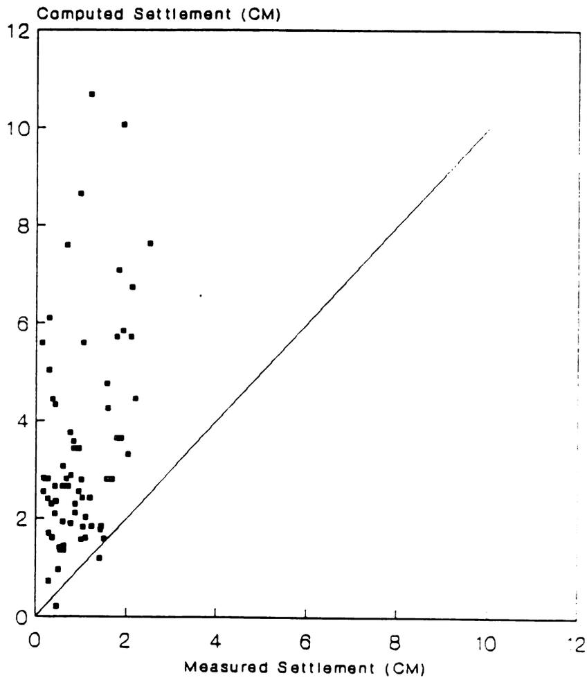
**Figure 25. Comparison Of Measured Settlements With Values Computed By Peck et al. Method**
