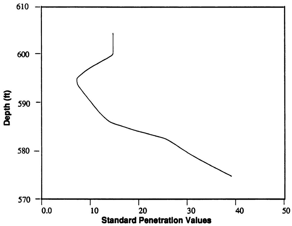
**Figure 14 . The Results of Standard Penetration Tests at the Site of MILL Building at Lake Michigan (after D'Applonia ,1968)**
