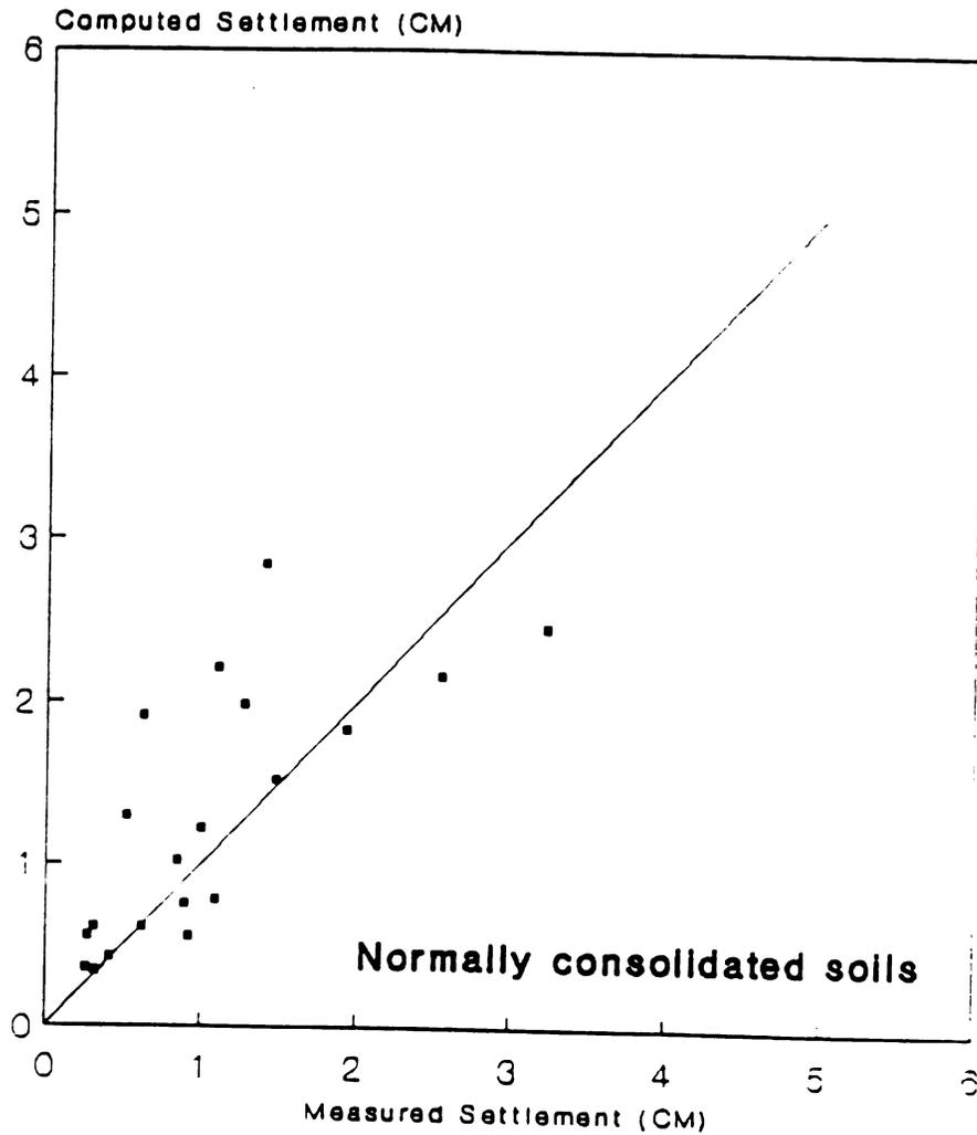
**Figure 12. Comparison Of Measured Settlements With Values Computed By Proposed Method**
