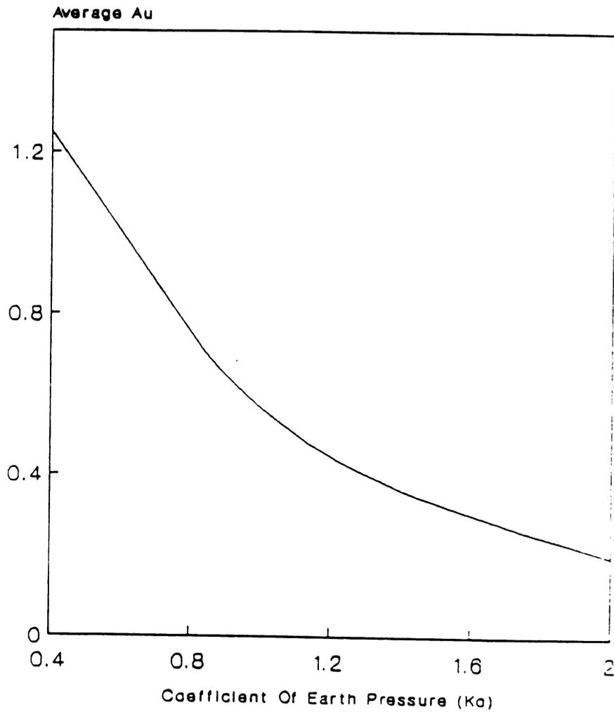
**Figure 11. Relationship Between Skempton's Pore Pressure Parameter And Coefficient Of Earth Pressure( Holtz,1978)**
