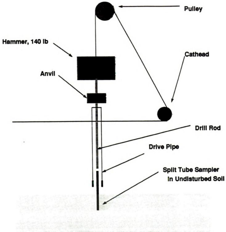
Figure 1. Schematic Diagram of Standard Penetration Test with Split Spoon Sampler
