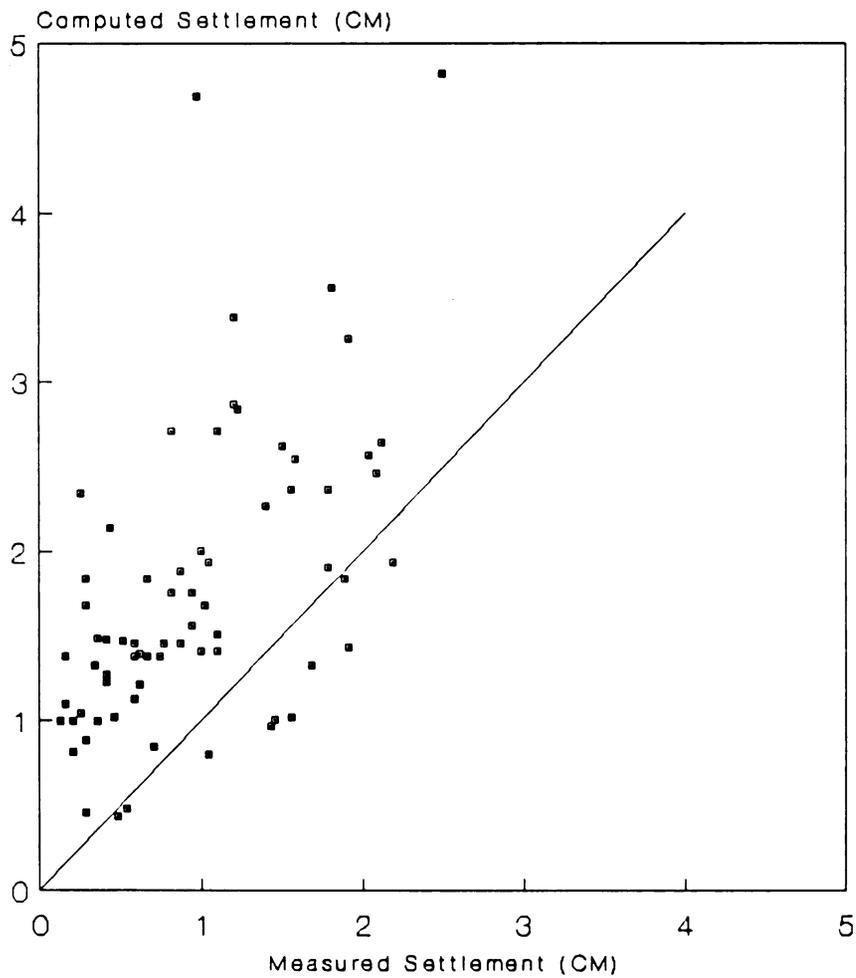
**Figure 23. Comparison Of Measured Settlements With Values Computed By Meyerhof Method**
