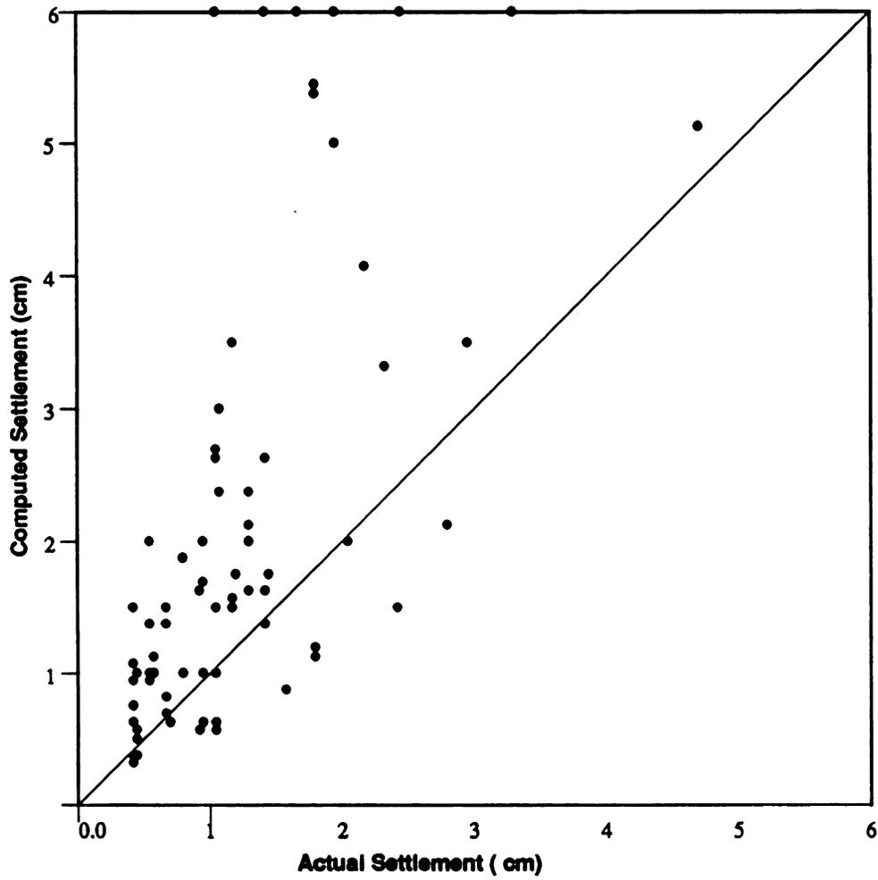
**Figure 8 . Comparison of Measured Settlements with Values Computed by Schmertmann's Method ( after, Jayapalan and Boehm, 1986 )**
