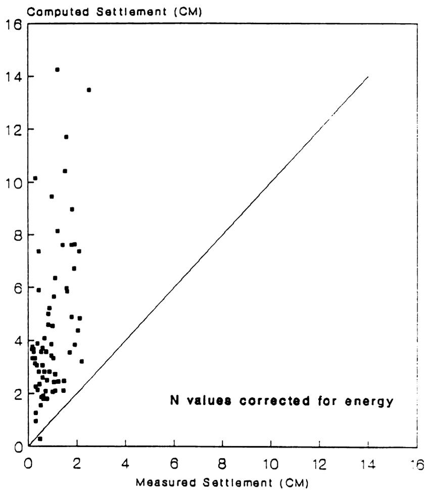
**Figure 30. Comparison Of Measured Settlements With Values Computed By Peck et al. Method**
