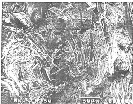
Fig. 8-J. Recycled HDPE (65%)/Wood Fiber (30%)/MA.PP (5%) composite. 350 magnification.
