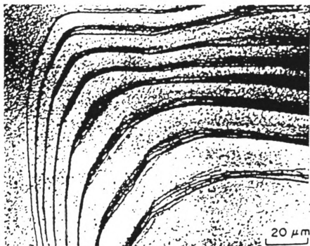
Fig. 8. Optical micrograph, using Nomarski interference contrast, showing the presence of a fine structure within the migration markings after testing for 8 cycles reverse bending at a frequency of 0.17 Hz and a strain amplitude of \pm 0.28\% [14,15].
