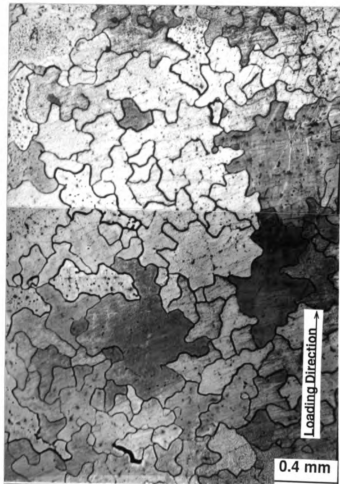
Fig. 27 Microstructure of Ni 3 Al, in the plane parallel to the loading axis, annealed at 800°C for 5 hour, after 100 cycles of 0.5% strain amplitude at 600°C.
