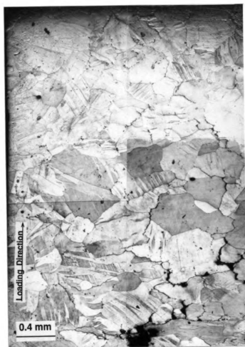
Fig. 28 Microstructure of Ni 3 Al, in the plane parallel to the loading axis, annealed at 1200°C for 2 hour, after 1000 cycles of 0.5% strain amplitude at 600°C.
