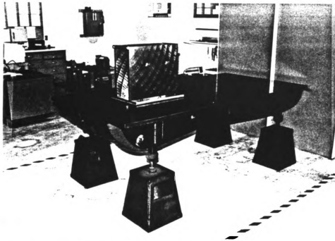
Figure 4.1. Static fixture for forearm testing.
