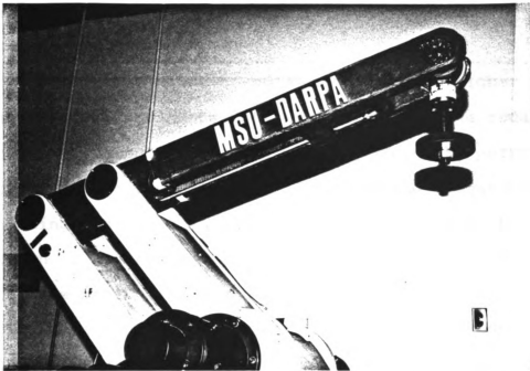
Figure 2.11. P-50 robotic manipulator with end-effector and payload.
