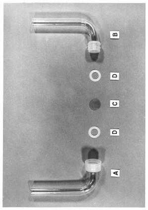
Figure 3. Set of assembled apparatus for the cuticular penetration studies.
