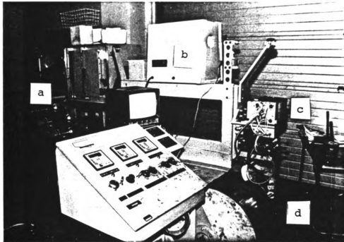
Figure III.2. Photograph of a prepregger machine manufactured by the Research Tool Company.
